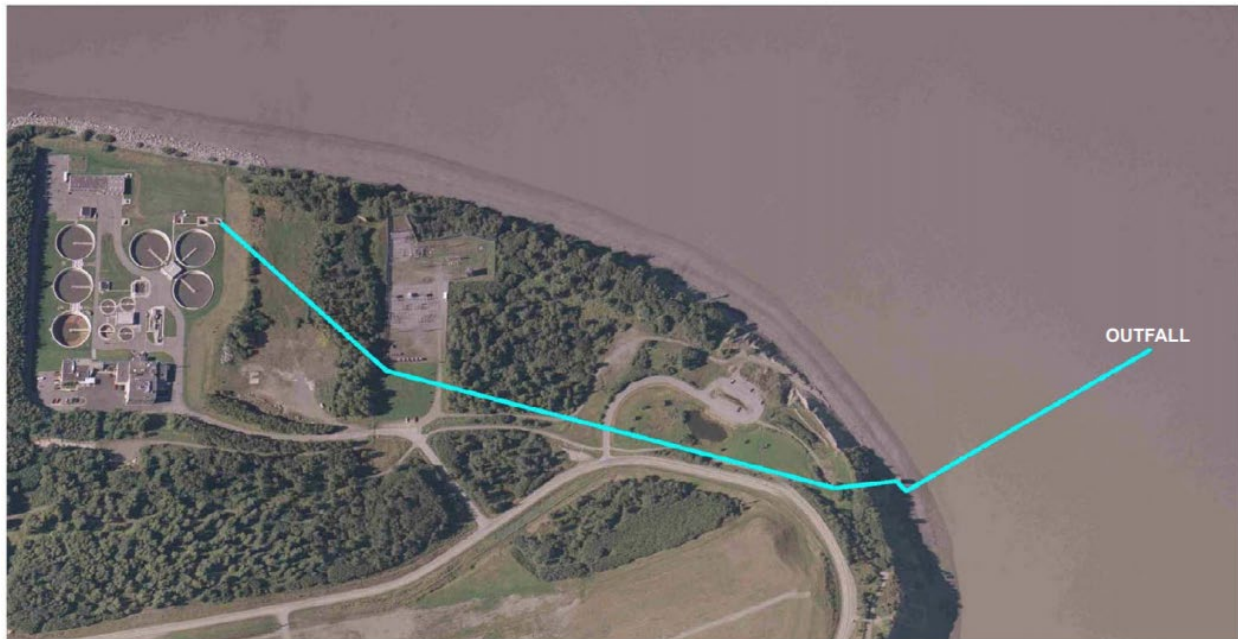
Figure 20. Route of outfall pipe for the Anchorage John M. Asplund Wastewater Treatment Facility.
