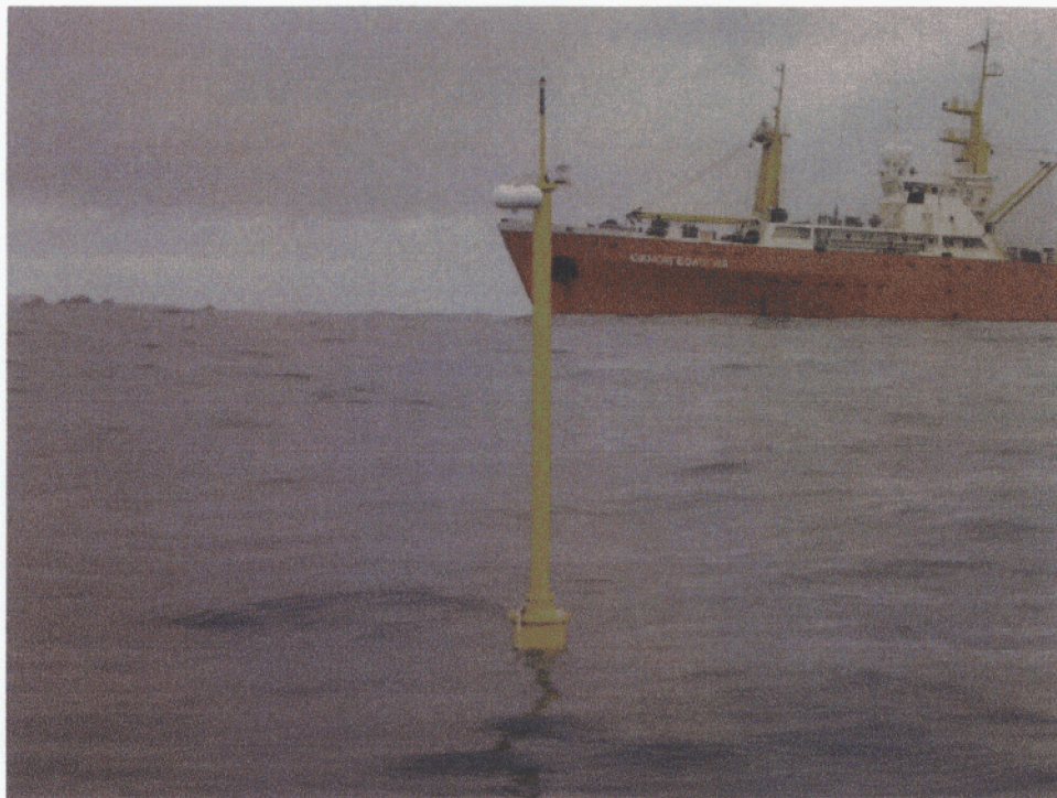
Figure 10.1. Multi-instrumented buoy deployed from R/V Yuzhmorgeologiya . The radar reflector, strobe and radio-modem antenna are visible at the top of the buoy's mast.
