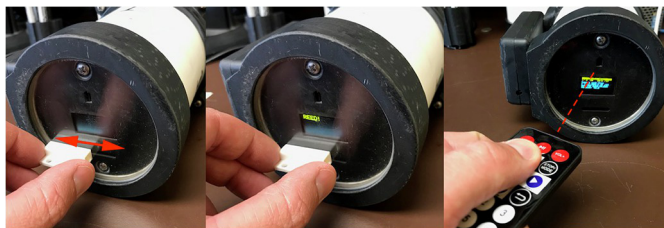
Fig. 8. Moving a magnet across the face of the reed switch will wake the SASE from sleep mode. With line of sight, the IR remote can be used to communicate with the IR receiver for navigating through the SASE menus.
