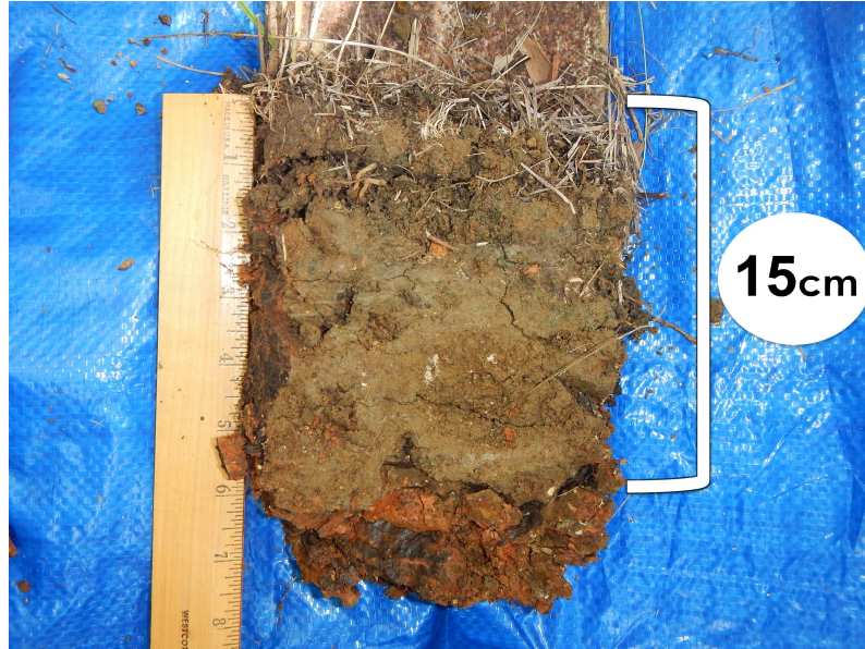
Figure 10. A soil profile removed from the ground used to confirm soil depth measurements taken with a soil probe. The top 15cm in the profile represents accumulated soil and detritus that deposited behind the sock. The soil profile displays a discontinuity at 15 cm depth and a shift to hardpan soil, or the pre-existing soil base.
