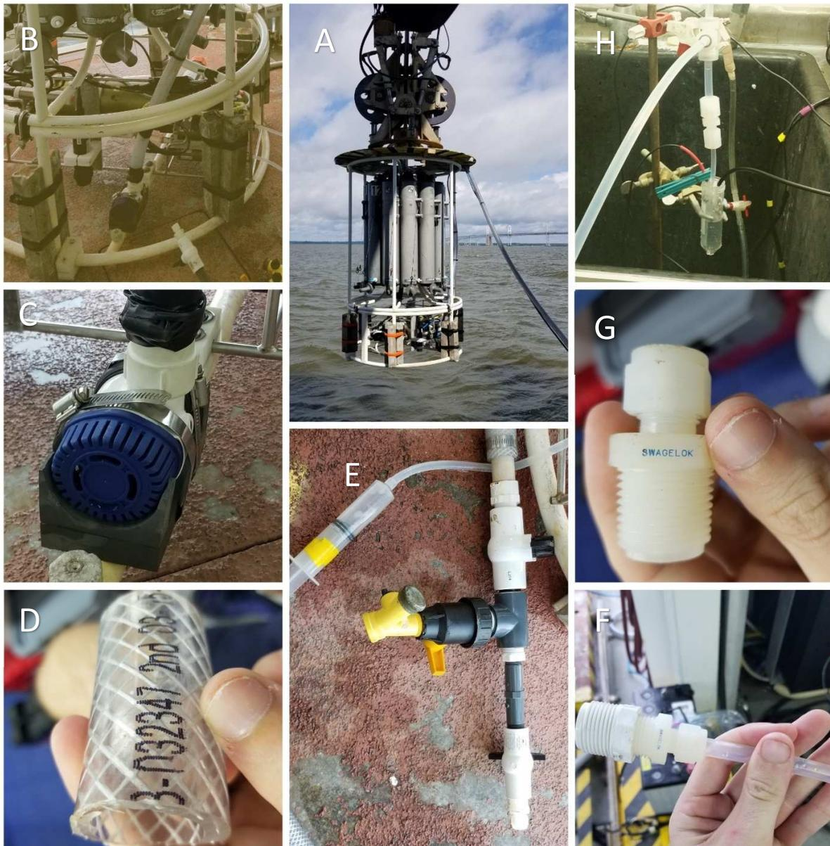
**Figure 1** A) The pump system is zip tied to the CTD rosette, with the bilge pump on the bottom. Tubing connects the structure to the onboard flow cells. B) A closer view of the bilge pump zip-tied to the bottom of the CTD rosette near other sensors. C) Bilge pump fastened to rosette. D) 1 3/8" tubing at sampling end attached to bilge pump E) T tube
