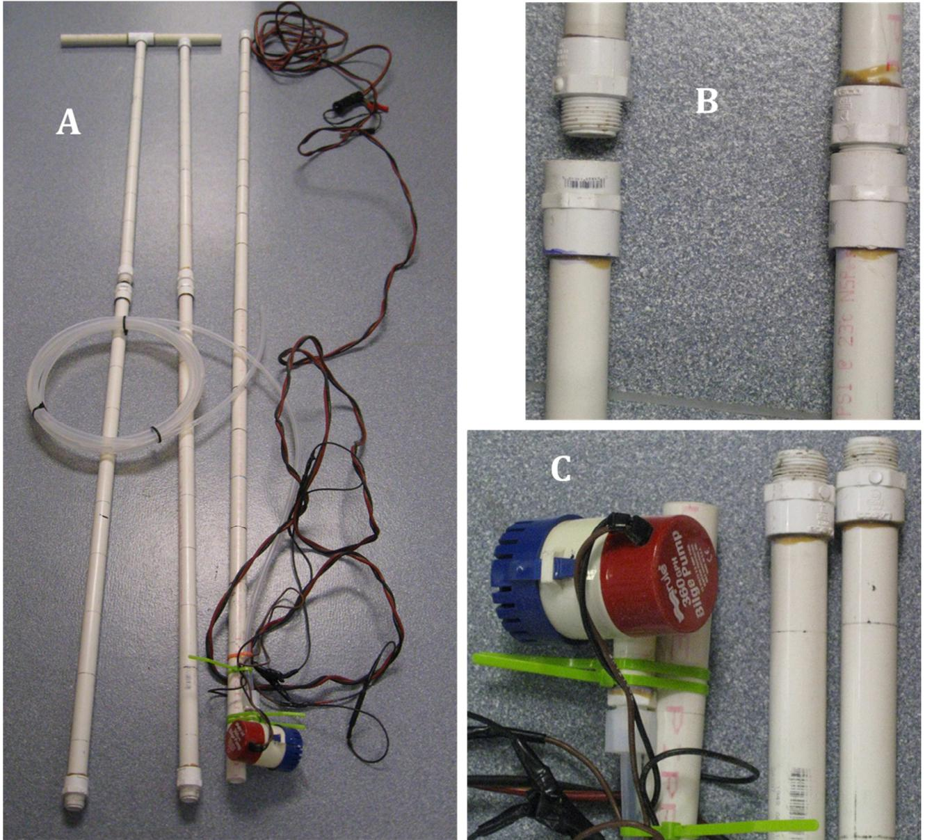
**Figure 5** A) Small boat pump profiler with 2, 2 meter extensions and 2,1 meter extensions.
