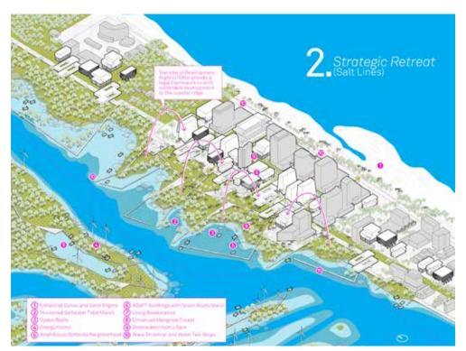
Figure 11. Axonometric of Strategic Retreat Scenario where re-development efforts and integration of green infrastructure are concentrated along highest elevation at coastal ridge and rewilding of lower elevation areas with natural landscapes.
