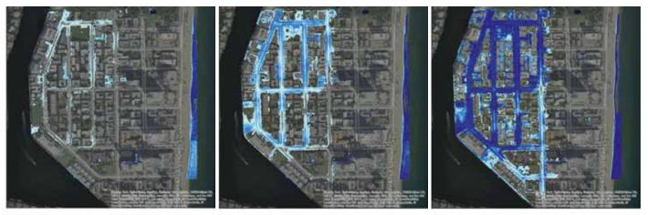
ONE-FOOT SLR At one foot of sea level rise streets to the west of the neighborhood become permanently flooded. The city is currently installing tidal valves and duckbills to prevent salt water from back-flowing into drainage infrastructure.
