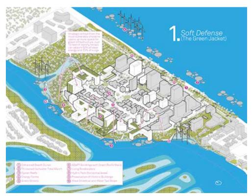
Figure 8. Axonometric of Soft Defense Scenario showing "Green Jacket," and green and blue streets.
