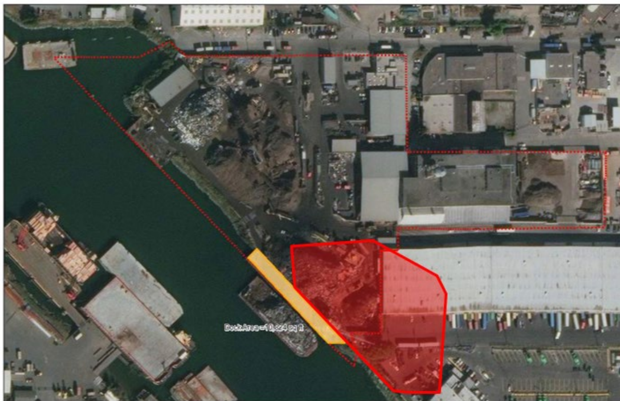
Figure 3. South dock to be replaced with material holding area (red) landward of the dock into which stormwater will be drained.
