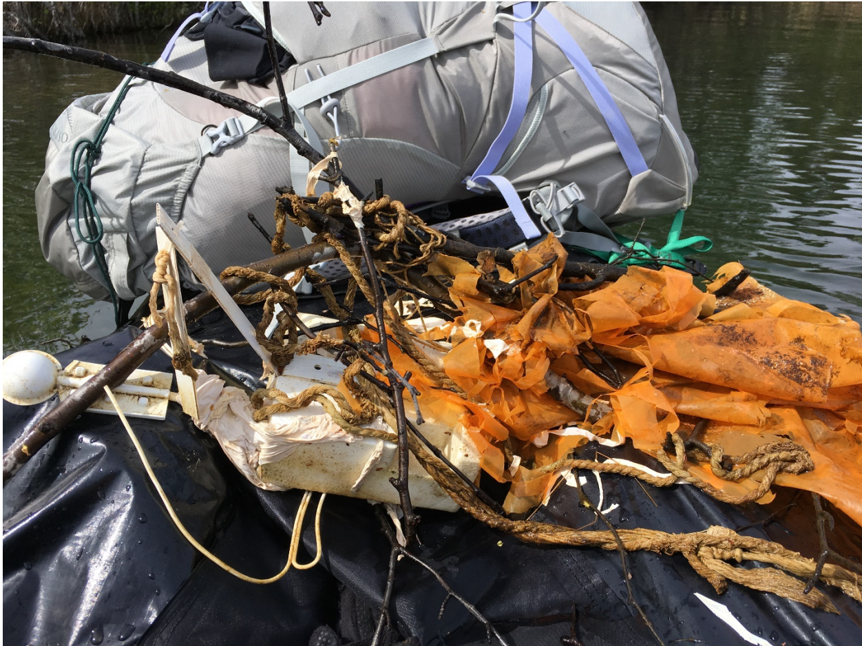
Figure 4. Example of a spent weather balloon retrieved from a lake in Alaska. The radiosonde was housed in the white Styrofoam container, the orange is the remains of the parachute, shards of the white plastic balloon can also be seen.
