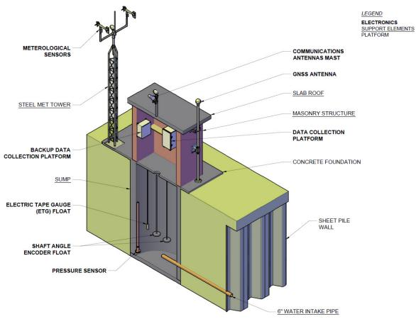
Figure 3. Typical Great Lakes gauge house and sump NWLON station
