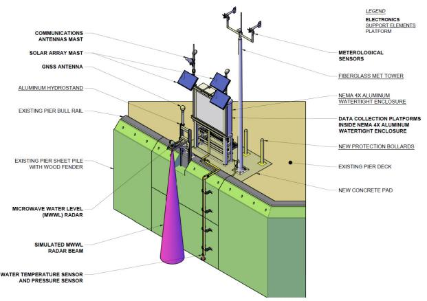
Figure 1. Typical coastal NWLON station configuration
