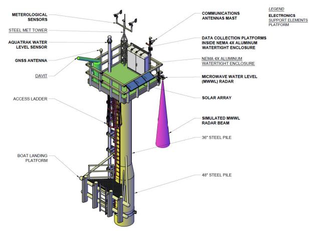
Figure 2. Typical nearshore NWLON station on a hurricane-hardened steel monopile
