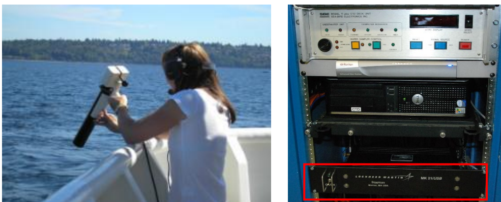
Figure 5. Sippican XBT launch from the aft deck (left). Deck unit for Sippican XBT (right).
