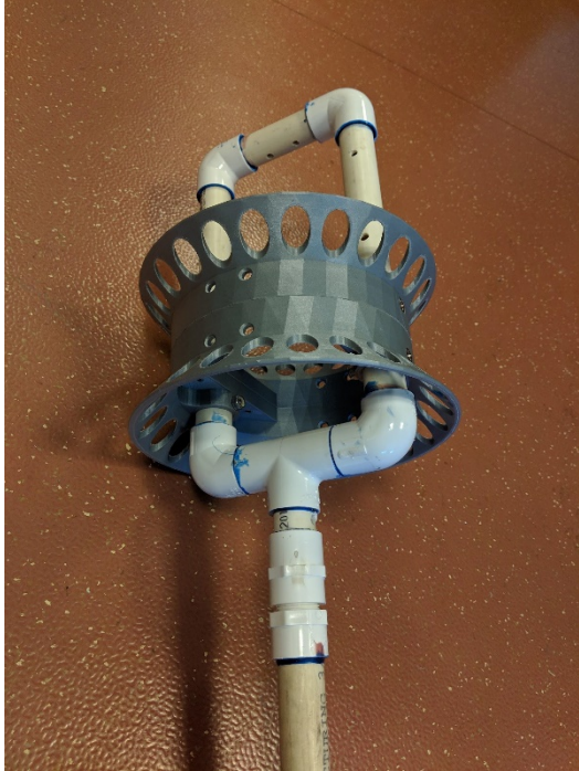
Figure 39. Image showing the construction of the drum using PVC pipe handles and a 3D printed drum.
