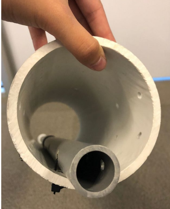
Figure 1. Image of the 0.75-inch PVC pipe attached to the drum using cable ties. The four holes to the right and left of the Schedule 80 pipe is where one of the two-pound weights will be attached.
