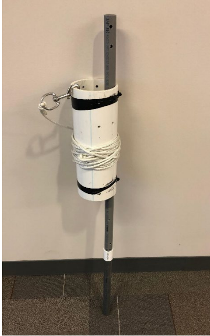
Figure 2: Example drum. The PVC pipe connected to the bottom of the male adapter (white PVC) may vary in size to ensure that the center of the drum reaches 1 min height. Electrical tape on the drum is used to cover cable tie ends.
