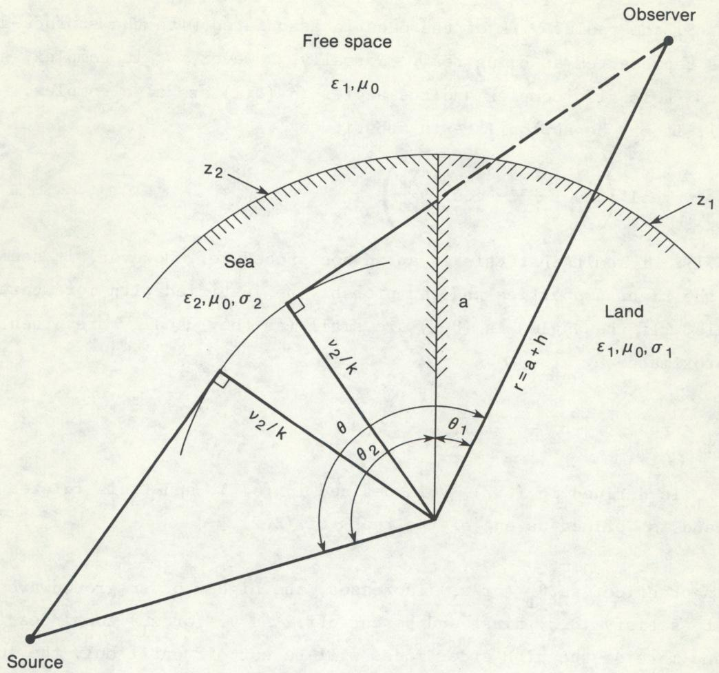
Figure 9. Geometry showing cut off of a sea-type groundwave mode for an elevated observer who is too far from the shoreline.
