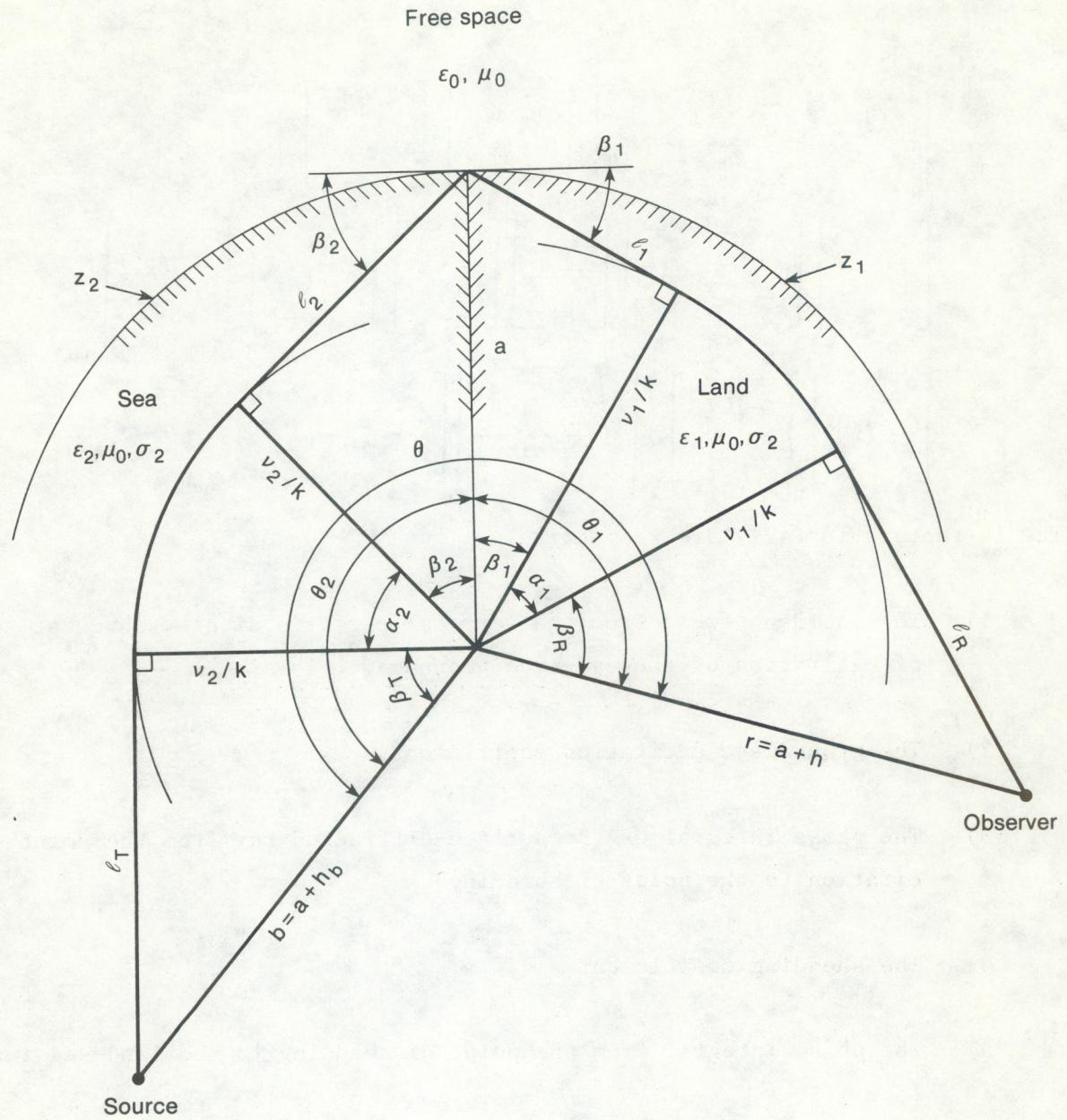
Figure 5. Geometry to represent coupling of groundwave modes at a land-sea boundary by edge-diffraction. Although the rays are unrealistically represented as being below the Earth's surface, the correct geometrical relationships allow this figure to be useful for making calculations.
