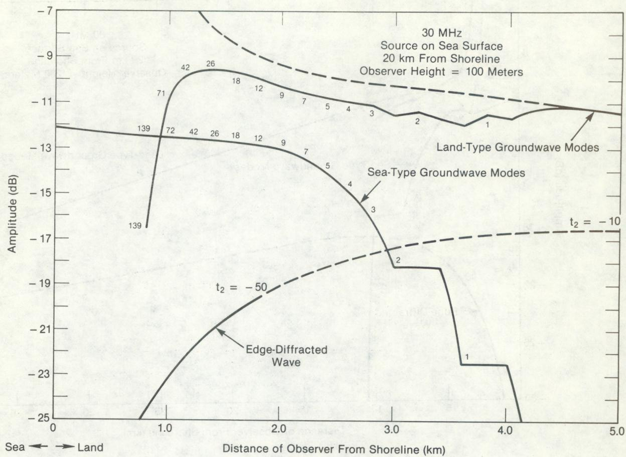
Figure 17. The field near the land-sea interface for an observer 100 m above sea level. The other conditions are the same as in Fig. 12.
