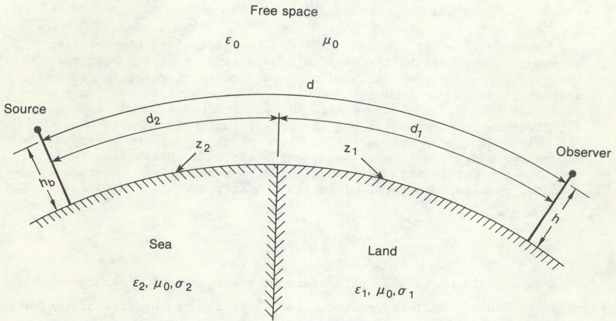
Figure 1. Geometry for propagation over a mixed land-sea path. The source is above the sea (characterized by a permittivity  $\epsilon_2$  and conductivity  $\sigma_2$ , or a surface impedance  $z_2$ ), and the observer is above land (characterized by a permittivity  $\epsilon_1$  and conductivity  $\sigma_1$ , or a surface impedance  $z_1$ ). The conductivity of free space is zero, and  $\mu_0$  is the magnetic permeability through the medium.
