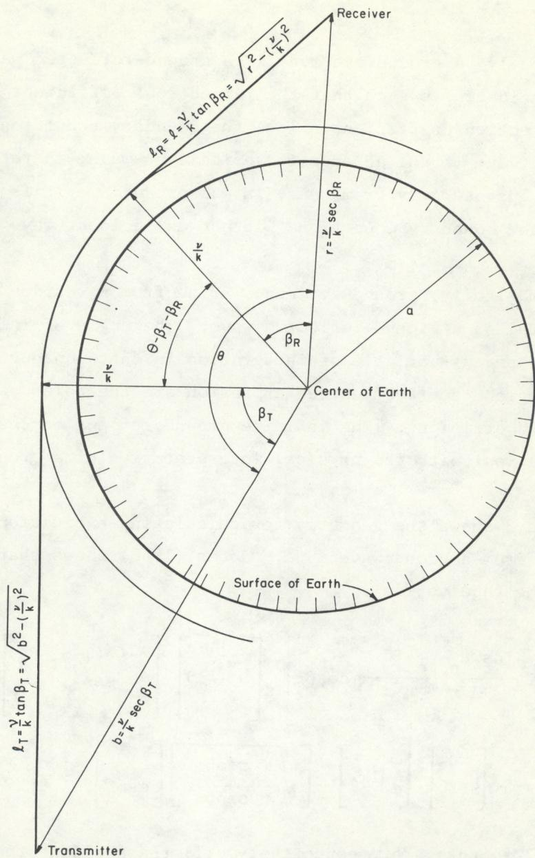
Figure 3. Representation of a groundwave mode by a surface-diffracted ray at a complex height  $v/k - a$ . The sphere of complex radius  $v/k$  is a caustic for the groundwave mode. From Jones (1968; Fig. 3).
