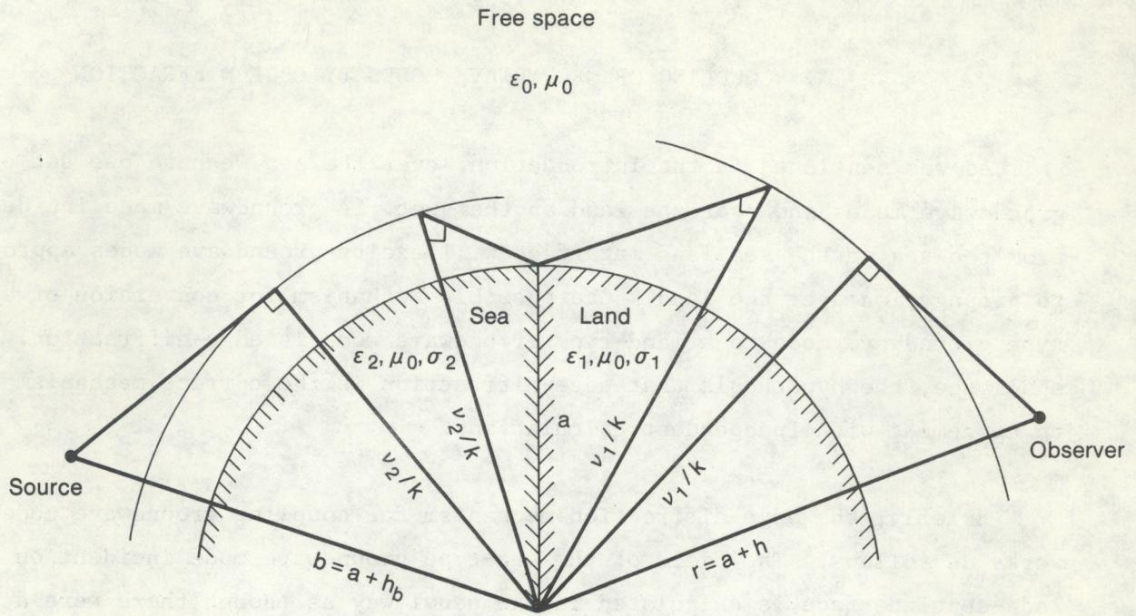
Figure 4. Geometry to represent coupling of groundwave modes at a land-sea boundary by edge-diffraction. The impossibility of drawing a ray from the land-sea interface that is tangent to the caustic for the groundwave mode disqualifies this figure as being useful for making calculations.
