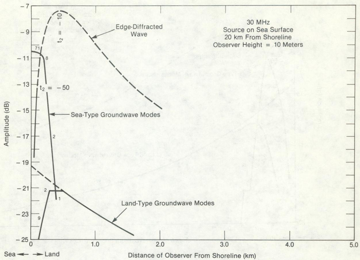
Figure 13. The field near the land-sea interface for an observer 10 m above sea level. The other conditions are the same as in Fig. 12.
