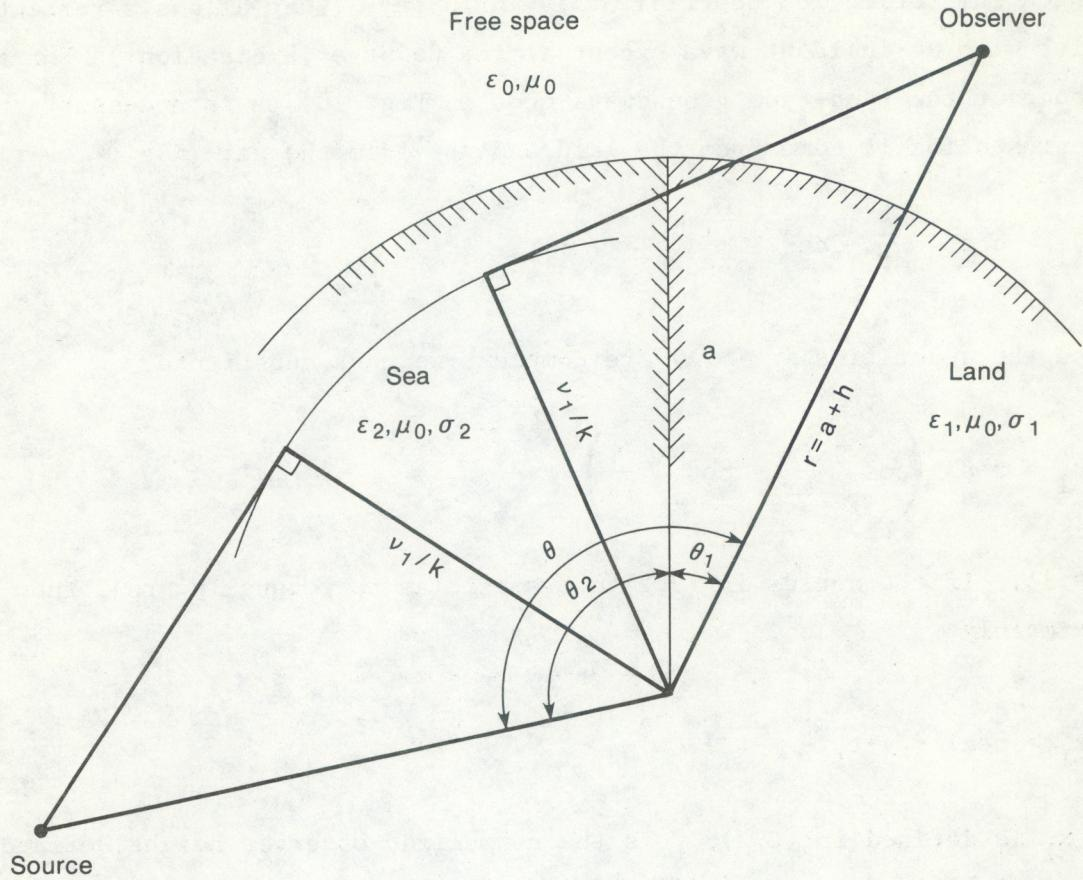
Figure 10. Geometry showing how the ray that represents a land-type groundwave mode propagates in a straight line from the Earth's surface to the observer. The ray must intersect the Earth's surface on the land side of the land-sea interface to satisfy the boundary condition (an infinite ground reflection coefficient) for a land-type groundwave mode.
