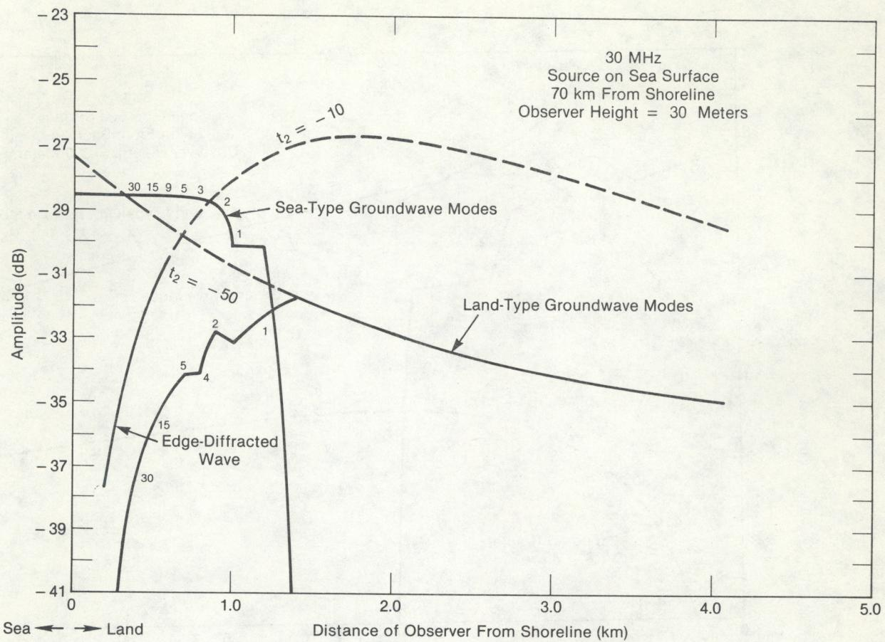
Figure 20. The field near the land-sea interface for an observer 30 m above sea level. The source is a vertical electric dipole on the surface of the sea 70 km from the shoreline. The other conditions are the same as in Fig. 12.
