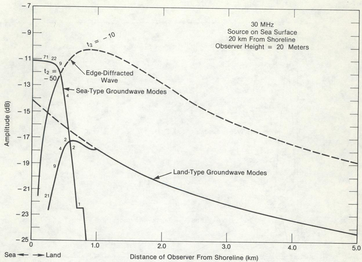
Figure 14. The field near the land-sea interface for an observer 20 m above sea level. The other conditions are the same as in Fig. 12.
