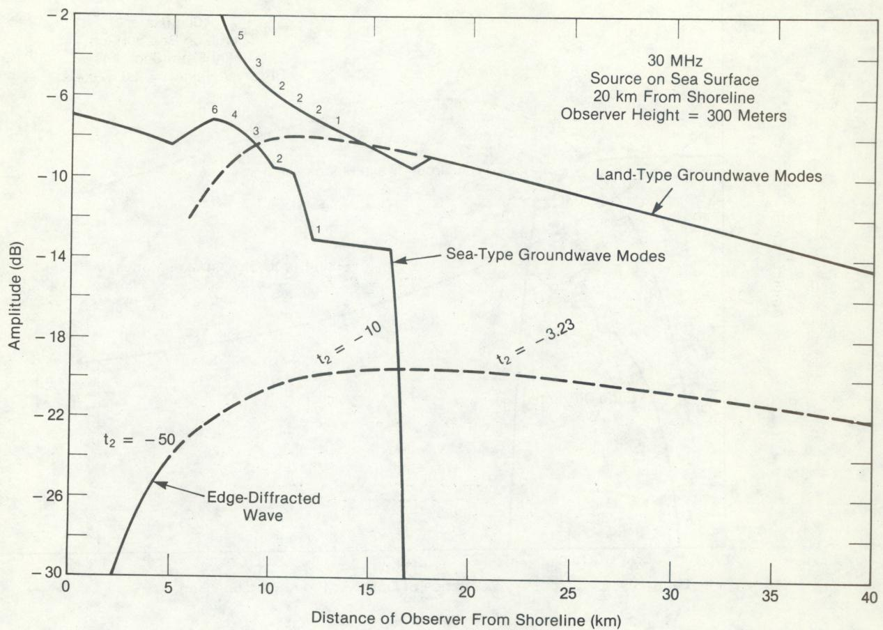
Figure 19. The field near the land-sea interface for an observer 300 m above sea level. The other conditions are the same as in Fig. 12.
