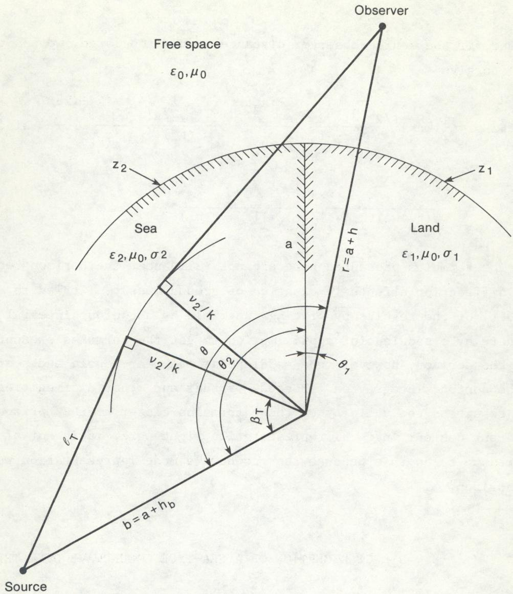
Figure 8. Geometry showing how a sea-type groundwave mode can be observed over land by an elevated observer.
