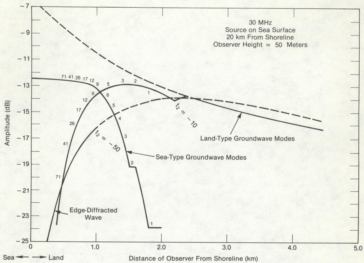
Figure 16. The field near the land-sea interface for an observer 50 m above sea level. The other conditions are the same as in Fig. 12.
