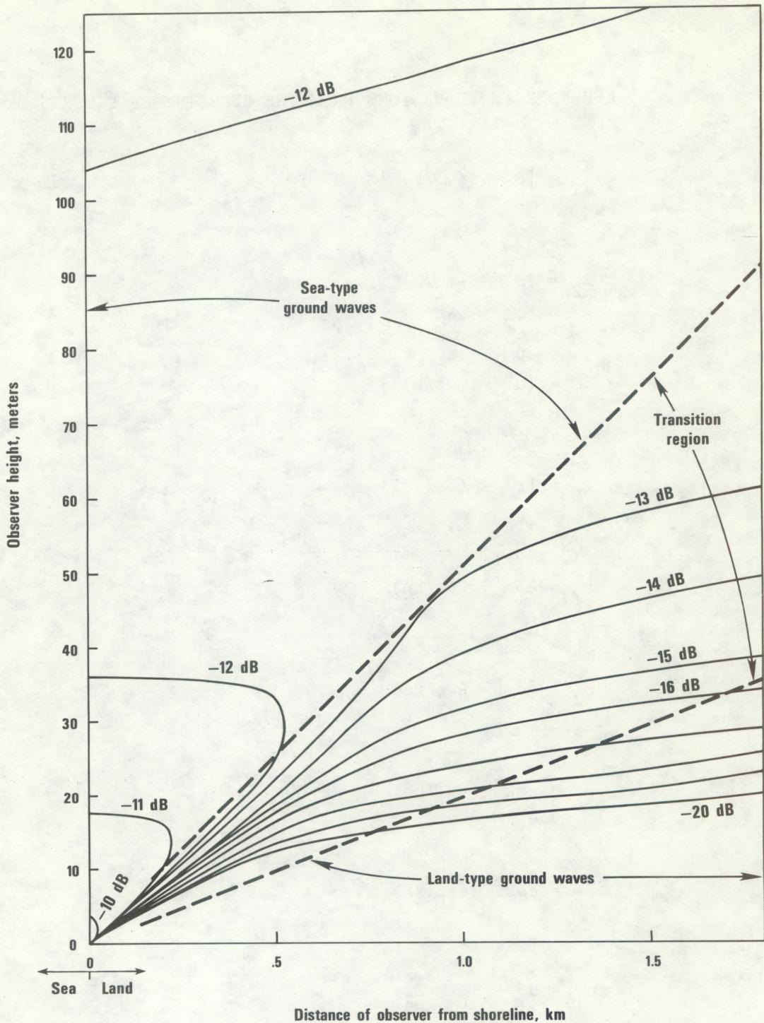
Figure 23. Contours of constant field strength over land near a land-sea interface, as in Fig. 21, but showing more detail near the shoreline.
