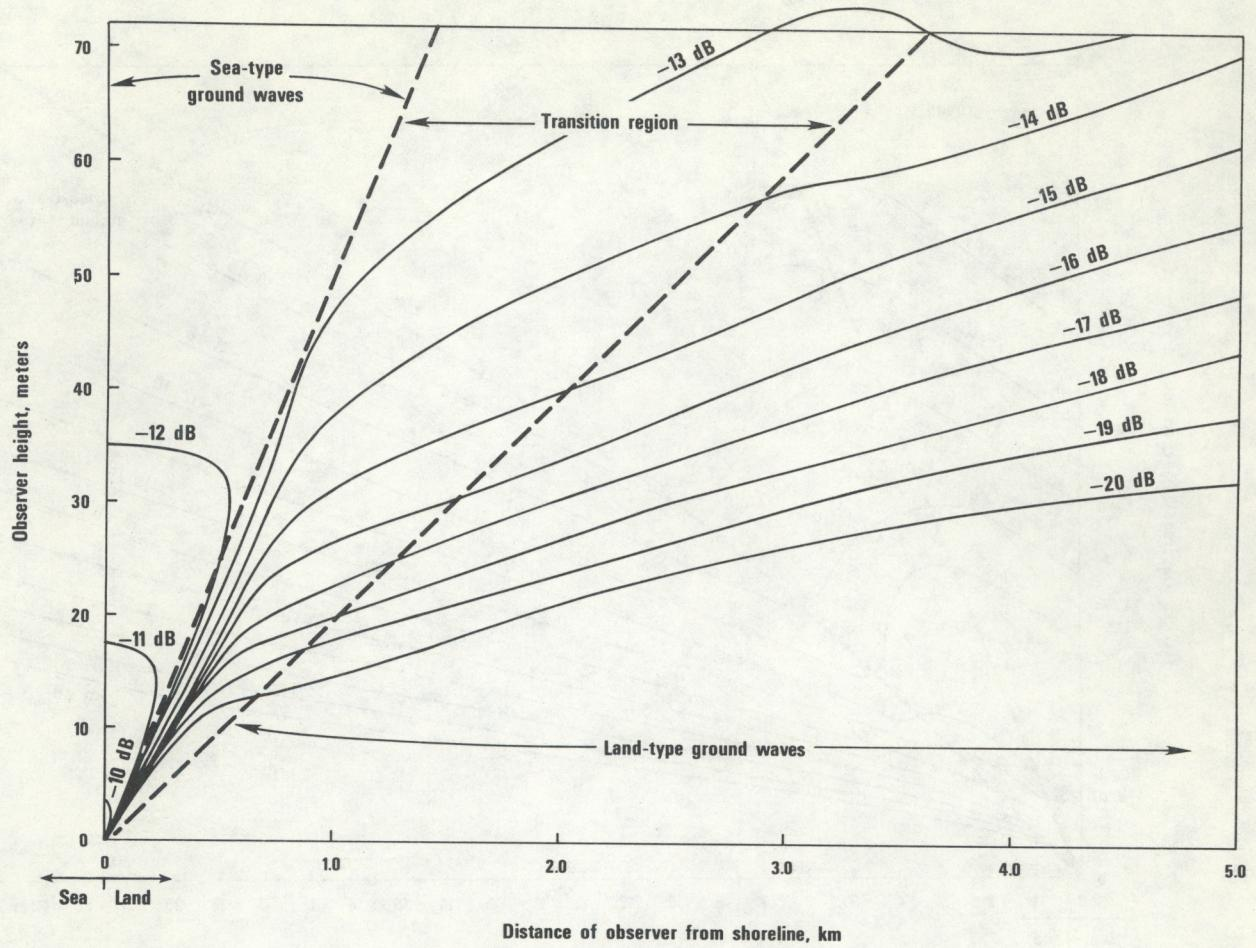
Figure 22. Contours of constant field strength over land near a land-sea interface, as in Fig. 21, but showing more detail near the shoreline.
