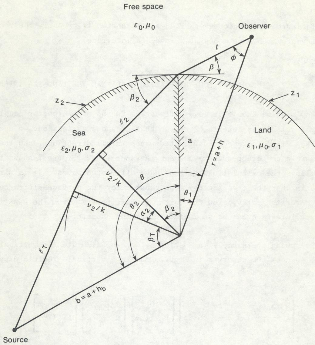
Figure 7. Geometry to represent excitation of an edge-diffracted wave by a groundwave mode incident on a land-sea boundary. One ray of the cylindrical edge-diffracted wave is shown.
