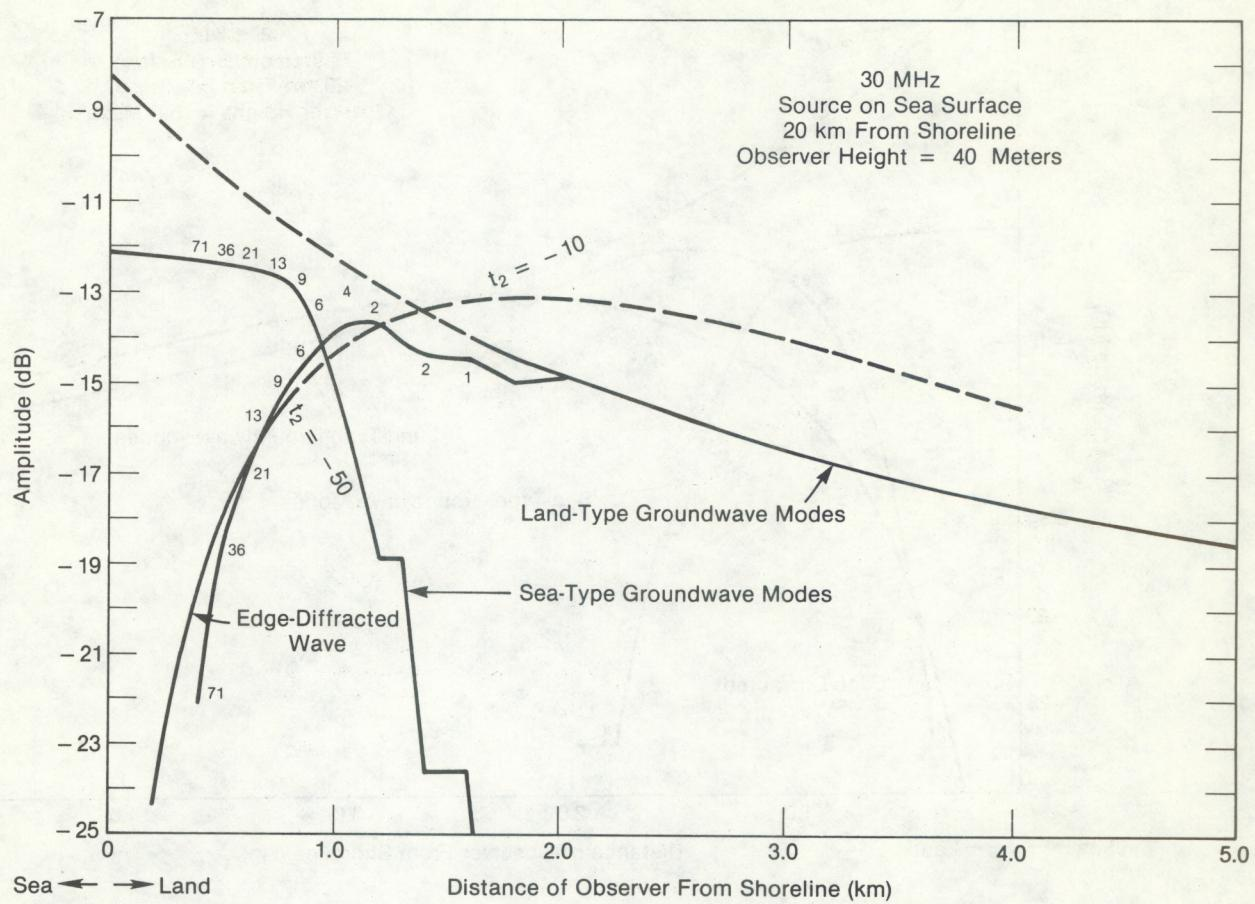
Figure 15. The field near the land-sea interface for an observer 40 m above sea level. The other conditions are the same as in Fig. 12.
