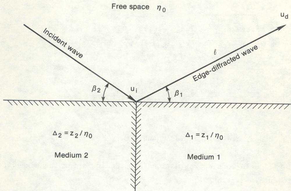
Figure 6. Geometry for edge diffraction at a land-sea interface. Each of the two lower media is characterized by a surface impedance  $z_2$  or  $z_1$ . We consider a plane wave to be incident on the land-sea interface. One ray of the cylindrical edge-diffracted wave is shown.
