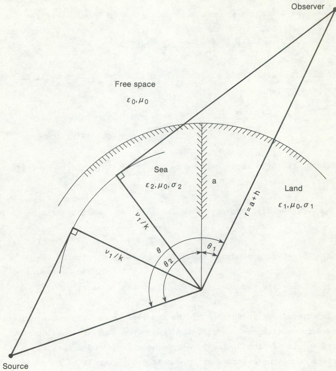
Figure 11. Geometry for an observer in the shadow zone of the land-type ground-wave mode that was excited at the land-sea interface. The ray that would connect the caustic of the land-type groundwave mode with the observer intersects the Earth's surface over the sea. At that point of intersection, the ray fails to satisfy the boundary condition (an infinite ground reflection coefficient).
