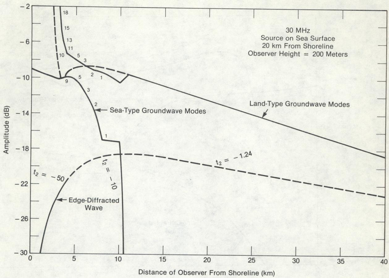
Figure 18. The field near the land-sea interface for an observer 200 m above sea level. The other conditions are the same as in Fig. 12.
