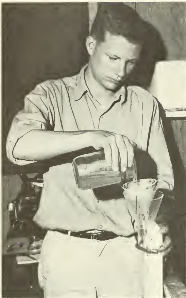
Figure 23.—Pouring plankton and preservative into draining cone is the third step of measuring plankton volume. The cone (333- \mu nylon mesh—see Table 1 for source of specifications) retains the plankton; the cylinder receives the fluid. Large sewing needles suspend cone in funnel keeping mesh from touching funnel's sides and allowing proper drainage.
