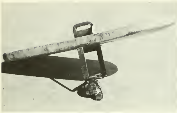
Figure 33.—Board used to calibrate T.S.-Flowmeters (one meter attached). The board is balsa wood, covered with fiber glass to make it waterproof, 4 ft long, 15 inches wide \times 2-1/2 inches thick (151.9 \times 38 \times 6.4 cm).
