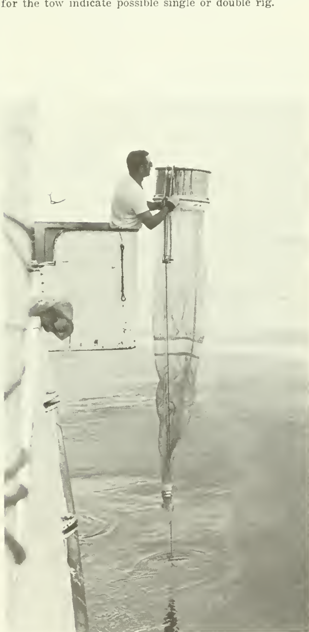
Figure 5.—Overside platform ("bucket") described in text, (also see Fig. 4 and 12), used to facilitate handling gear over water and away from side of ship. (The net is the Soutar-Hemingway Animal Trap (SHAT) used for vertical tows; it is not used or described here for standard collections for CalCOFI egg and larva data.)
