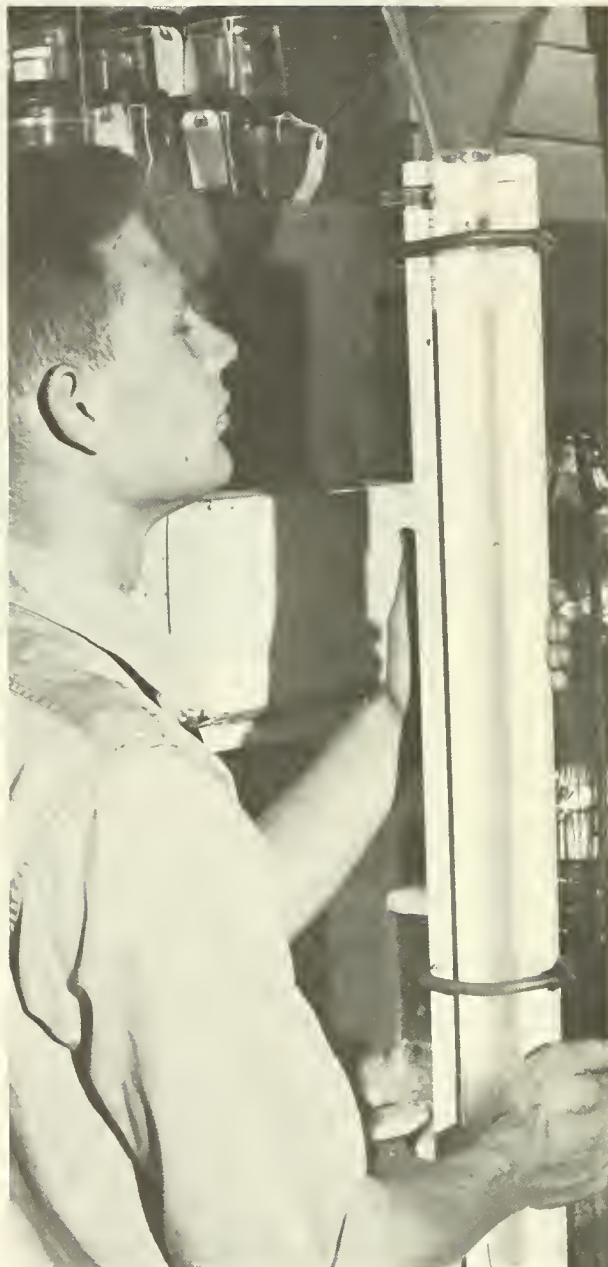
Figure 24.—Reading volume is the fourth step of measuring plankton preservative after plankton has drained to an occasional drop. The volume of the calibrated jar, holding plankton and preservative (Fig. 20), less the volume in the cylinder equals the displacement volume of the plankton. The cylinder is plastic tubing, 1-1/2 inches I.D. \times 34 inches long (3.8 \times 86.4 cm) with graduations etched on the cylinder or on a grooved board, as illustrated. The graduations on cylinder or on the board are 5-ml units from 0-600 ml and 2-ml units from 600-910 ml. Volumes are read to the nearest millimeter.
