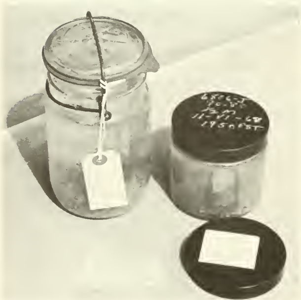
Figure 18.—Labels for plankton samples. Clockwise from upper left—Tie-on cardboard label on 1-quart (1 liter) bail-type jar; screw-on cap labeled with Martek pen, on 1-pint (1/2 liter) jar; self-adhesive label on screw-on cap; inside label on which information duplicates (not in any of these cases) whatever is written on an outside label. Inside label is made of 32-lb., chemically resistant linen called "Resist-all."
