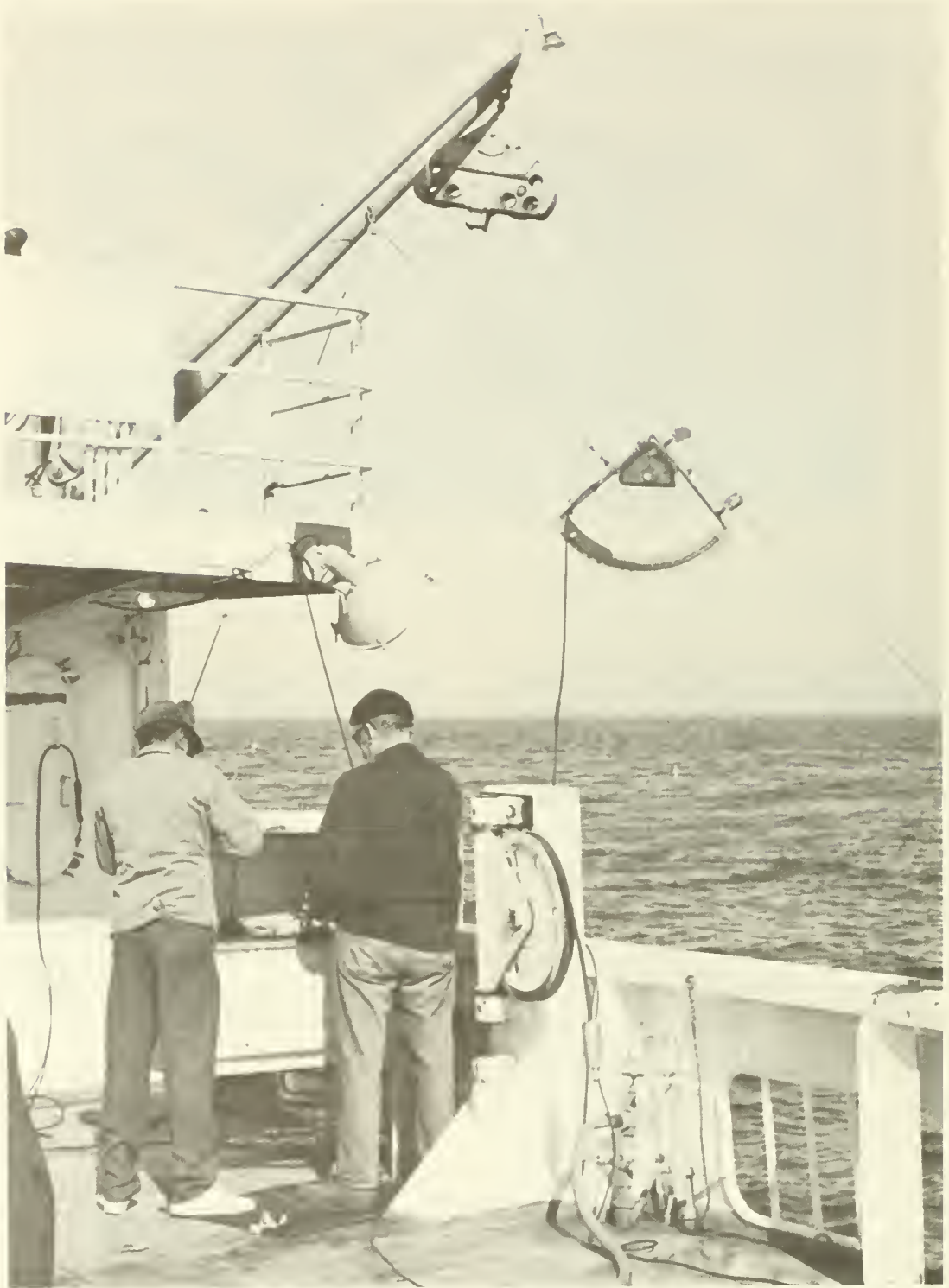
Figure 3.—View of boom and block, upper left (also see Fig. 2), on R/V Jordan. Plankton net tow in progress. Telemetering inclinometer (see also Fig. 8 and 9), used to indicate wire angles, hangs from towing wire. Slack in wire indicates that the net is being lowered. Man on right is the winch operator at winch console, close to rail where he can watch net operations during launching and retrieval. Man on left will record wire angles when net is retrieved (see plankton tow procedure).
