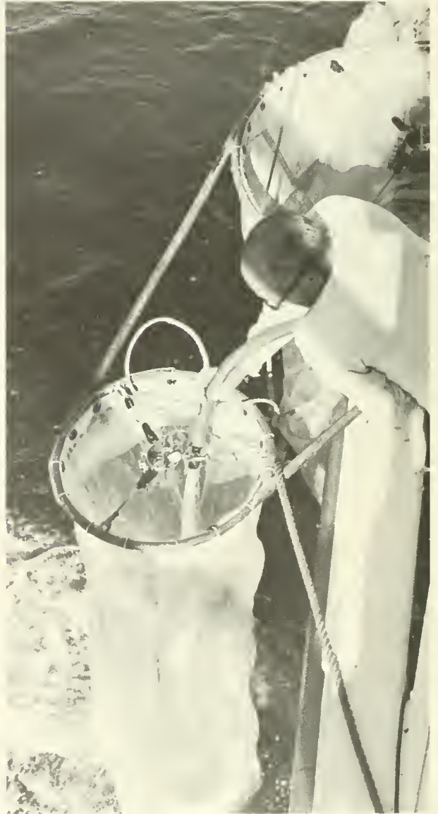
Figure 15.—Rinsing down plankton after net tow, before removing cod end with sample. Note: Cod end should be removed after it is hung from the ship's rail as shown in Figure 6.
