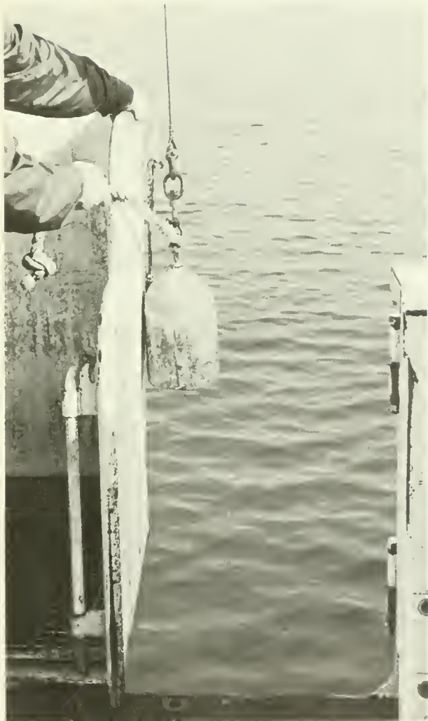
Figure 4.—Weight (100 lb. = 45 kg) being swung over-side at end of towing cable. The weight is a cast-iron tapered cylinder 7\frac{1}{2} inches (19.0 cm) in diameter, 13 inches (38 cm) high with its taper beginning about 9 inches (22.8 cm) from the bottom. One-inch (2.54 cm) stock is anchored in the casting and an eye, 1\frac{5}{8} -inch (4.5 cm) I.D., of the same stock is welded to it. After casting, the unit is heavily galvanized. The diameter of the eye is enough to take a strong shackle and a heavy line through it. Note swivel between the shackles which keeps the weight from twisting the wire. Casing, partially shown at lower right, is used to store the weight when not in use. Overside platform at left (also see Fig. 5 and 12) shows grill floor (description in text).
