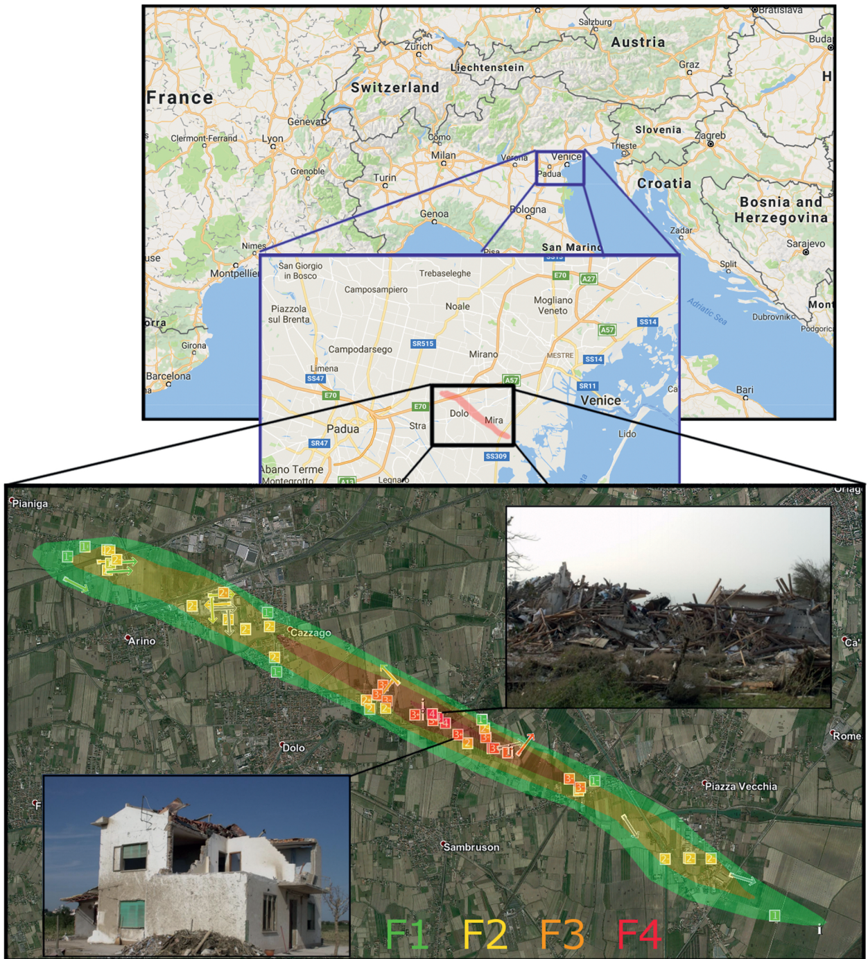
FIG. 9. Damage path of the violent tornado that occurred on 8 Jul 2015 near Dolo and Mira, Italy. Individual numbers indicate ratings of damage on the Fujita scale according to the procedure outlined by Feuerstein et al. (2011). The top-right damage photo inset shows the remains of the eighteenth-century Villa Fini. [Damage photos courtesy of A. Gobbi, MeteoNetwork Association. Map imagery courtesy of Google. Map data courtesy of GeoBasis-DE/Federal Agency for Cartography and Geodesy (Bundesamt für Kartographie und Geodäsie; BKG), Frankfurt, Germany; Google; Instituto Geográfico Nacional, Madrid, Spain; Mapa, GISrael, Tel-Aviv, Israel; and ORION Middle East (ORION-ME), Beirut, Lebanon.]
