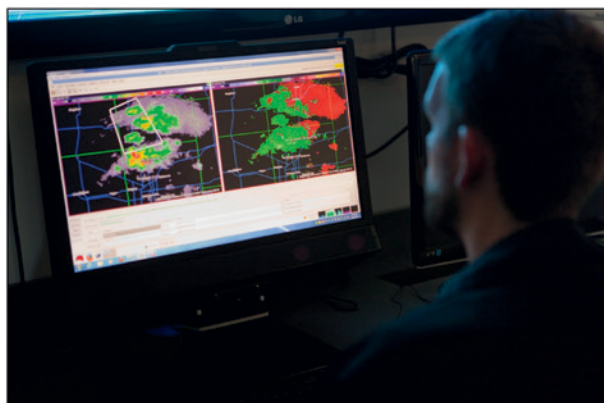
FIG. 1. Forecaster interrogating 1-min base velocity and reflectivity phased array radar data using the Warning Decision Support System-Integrated Information. The Tobii TX300 eye tracker is positioned below the monitor.
