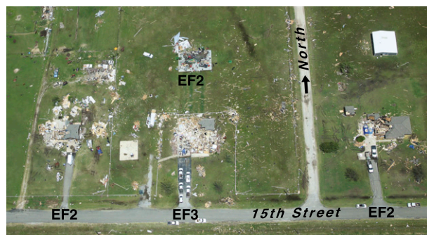
FIG. 12. An aerial photo looking north of a region depicting EF2 and -3 damage associated with the El Reno tornado. The location of the photo (shown in Fig. 11a) is \sim 500 m east of the intersection of Highway 81 and 15th Street.
