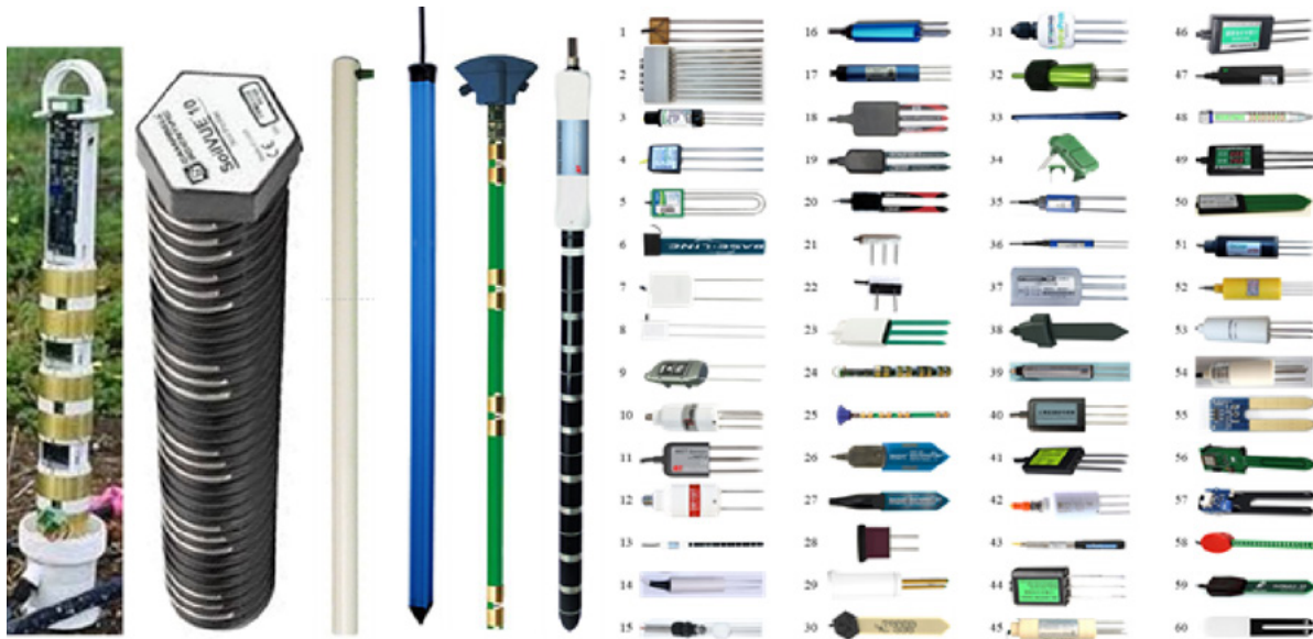
Figure 4.9: Array of electromagnetic-based bore-hole (left) and insertable soil water content sensors.
