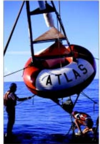
*Ocean Acoustic Monitoring System. Left to right: Hydrophone is deployed from the French vessel Le Suroit. The mooring is designed to place the hydrophone within the oceanic sound channel. NOAA and French researchers acoustically interrogate the newly deployed mooring to refine its position.*
