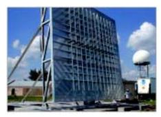
OAR - ETL - 449 Radar 449 MHz Wind Profiling Radar
