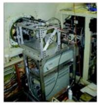
OAR - ETL - ABAEL **Airborne Aerosol Lidar** ABAEL uses backscatter lidar for aerosol detection via aircraft platforms.
