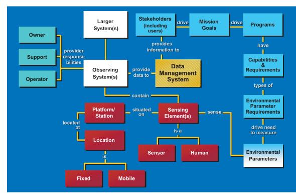
**Figure 7.** NOAA Observing Systems Architecture Relationship Diagram. The diagram entities are color coded by functions. Blue refers to the user requirements functional components. White refers to the observation functional component and its linkage to partner functions. Red refers to the observation system subcomponents. Yellow refers to the data management functional component, which includes the flow of information among all entities. Green refers to the observing system provider functions.
