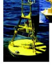
Examples of 6-meter boat-shaped buoy and 3-meter discus buoy.
