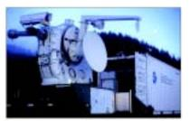
OAR - ETL - NOAA/K Mobile Scanning Cloud Radar NOAA/K is a dual-polarized, scanning, Doppler radar (short wavelength, 8.66 mm/35GHz), for cloud physics research and climate studies.
