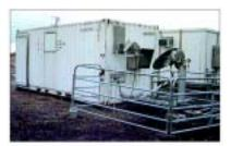
**OAR - ETL - Radiometer Container** This is a container fitted with microwave and infrared radiometers for the study of clouds.
