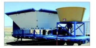
OAR - ETL - Wind Profiler - RB Electronically-Stabilized Wind Profiler This is a 915-MHz clear-air radar used for measuring wind speed and direction from 150 - 3000 m altitude. This system automatically compensates for platform motion.
