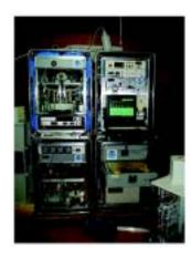
OAR - CMDL - AERO Aerosol System The purpose is to measure aerosol optical properties as a function of size and wavelength at baseline and regional stations.
