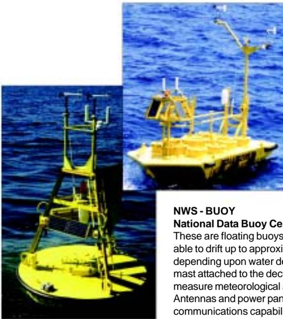
*Examples of 6-meter boat-shaped buoy and 3-meter discus buoy.*
