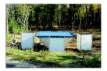
OAR -ETL- Profiling Radar -Tethered Aerostat Radar System This is a wind and temperature profiling radar operating at 449 MHz.
