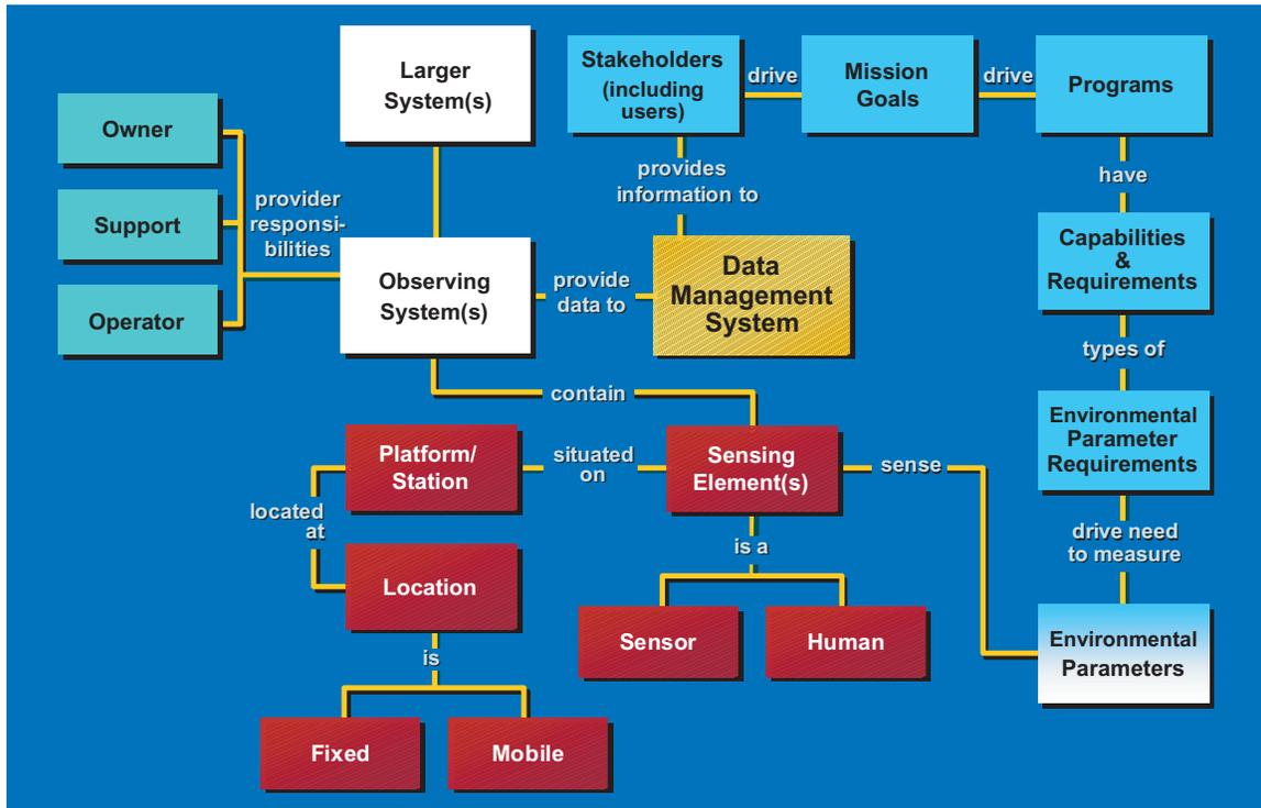
**Figure 7.** NOAA Observing Systems Architecture Relationship Diagram. The diagram entities are color coded by functions. Blue refers to the user requirements functional components. White refers to the observation functional component and its linkage to partner functions. Red refers to the observation system subcomponents. Yellow refers to the data management functional component, which includes the flow of information among all entities. Green refers to the observing system provider functions.
