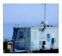
OAR - ETL - Lidar - MOPA - ost Dual Wavelength Doppler Lidar Mini-MOPA is a scanning Doppler lidar used in field campaigns to study atmospheric phenomena in the boundary layer.
