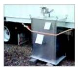
OAR - ETL - IR Radiometer OAR - ETL - Narrow Band IR Radiometer This is an infrared radiation sensor for measuring temperature.
