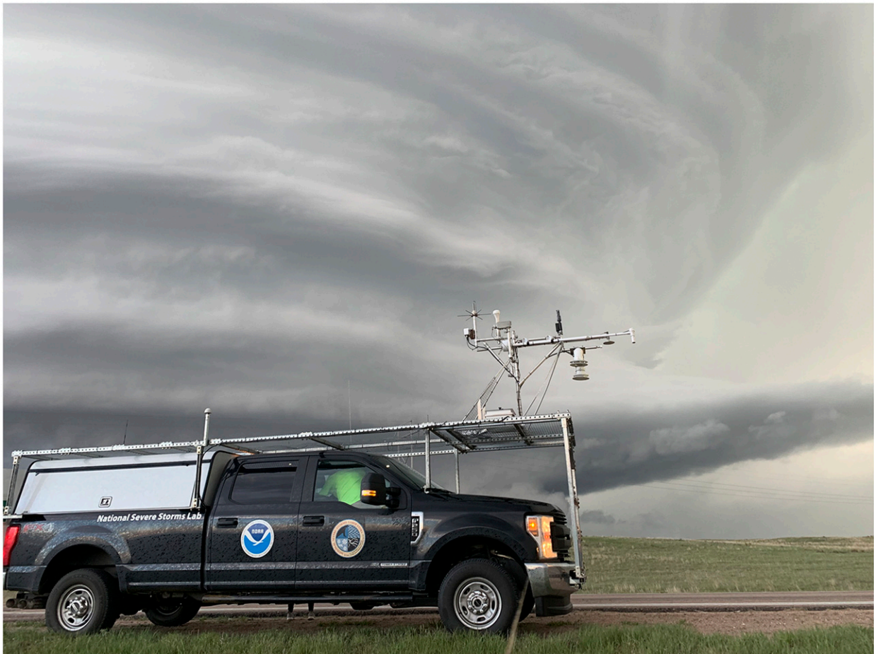
FIG. 6. A mobile mesonet vehicle in use during the Target Observations by Radars and Unpiloted Aerial Systems (UAS) in Supercells (TORUS) project in 2019. The U-tube can be seen on the front portion of the instrument rack, mounted above the front end of the truck.
