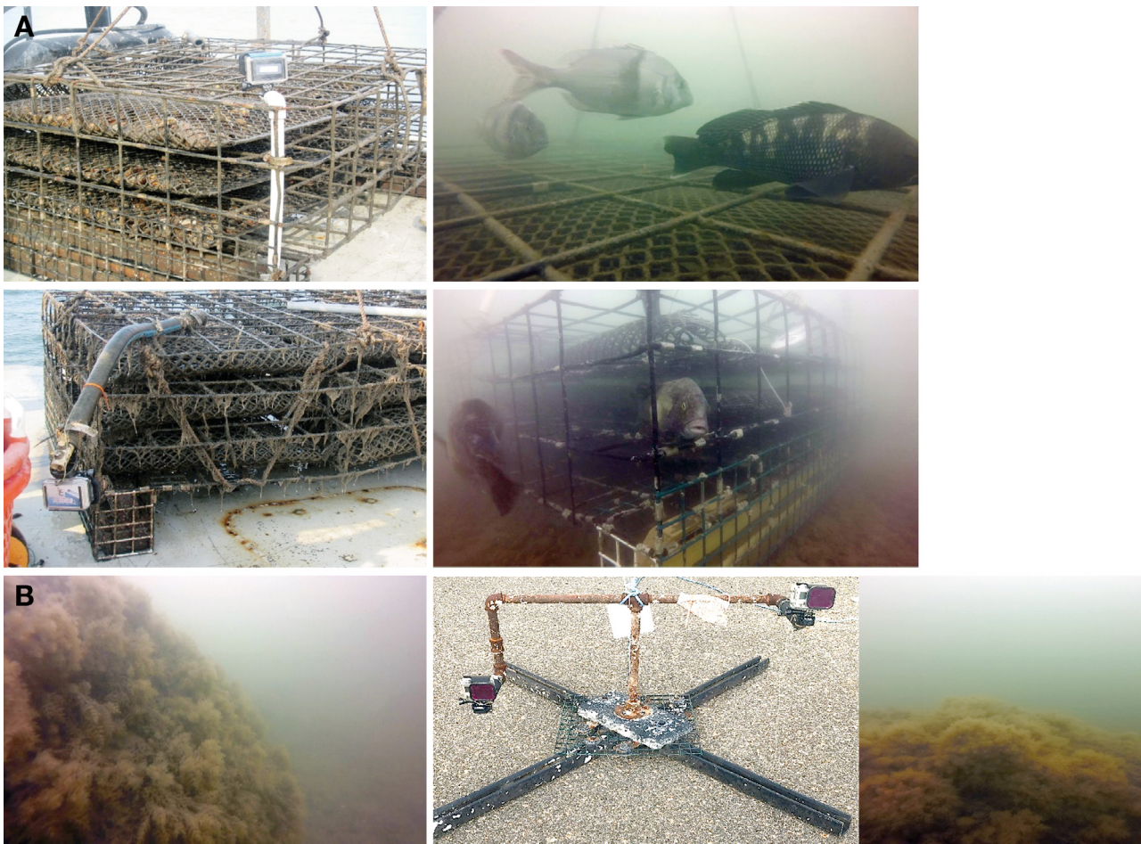
Fig. 2. Camera deployment and example video frames. (A) Two cameras were directly attached to the shelf-and-bag style oyster aquaculture cages; one showed images across the cage top, the second showed 2 sides of the cage and the cage-seafloor interface. (B) Two cameras were attached to minimal-structure 'T-platform' stands that were deployed adjacent to boulders on a rock reef; one showed images across the boulder top, the second showed the boulder side and boulder-seafloor interface
