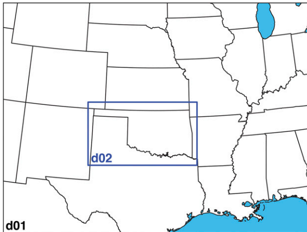
FIG. 9. Domain layout for the numerical simulation experiment. The horizontal grid spacings for domains 1 (black outline) and 2 (blue outline) are 3 and 1 km.
