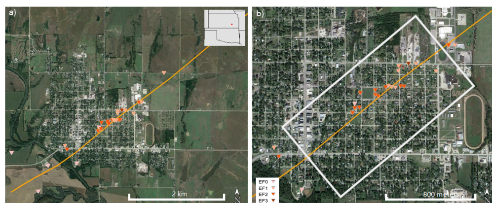
Figure 1. Kansas tornado, 26 June 2018 Eureka, (a) path overview and (b) survey site outlined in white box. Inverted triangles correspond to Enhanced Fujita (EF) scale ratings with the strongest damage (EF3) shown in dark red and weakest damage (EF0) shown in light pink were obtained from ground surveys conducted by the National Weather Service Weather Forecast Offices (NWS WFOs) Wichita, Kansas.
