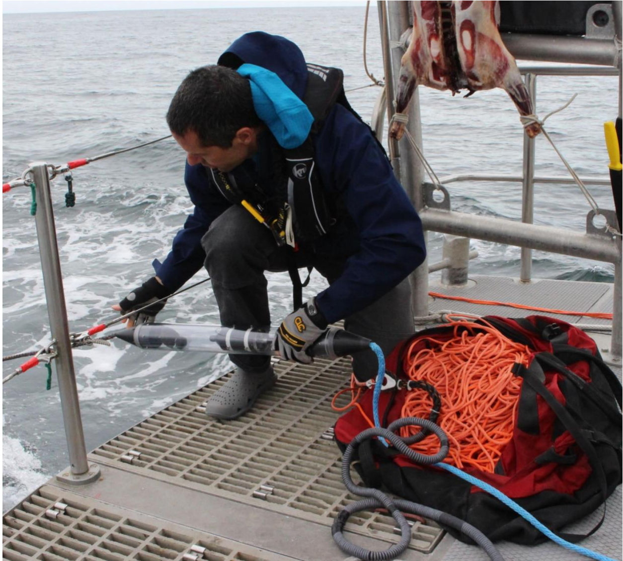
Figure 2. Deployment of a towed autonomous recording system with a single-channel SoundTrap ST300 recorder. The forward section of the head line (blue Dyneema line) is wrapped with 3/16" lead wire for weight. The towline is 1200' of 3/16" orange Dyneema.
