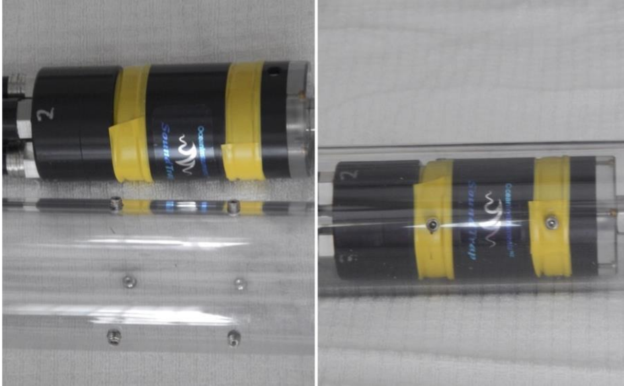
Figure 5. Set screws for securing the SoundTrap in the polycarbonate tube shown in the out position (left panel), SoundTrap with a strip of 1/8" open-cell neoprene filling the circumferential grooves and covered with yellow electrical tape (left and right panels), and SoundTrap installed in a towing position with the set screws flush with the exterior of the tube (right panel).
