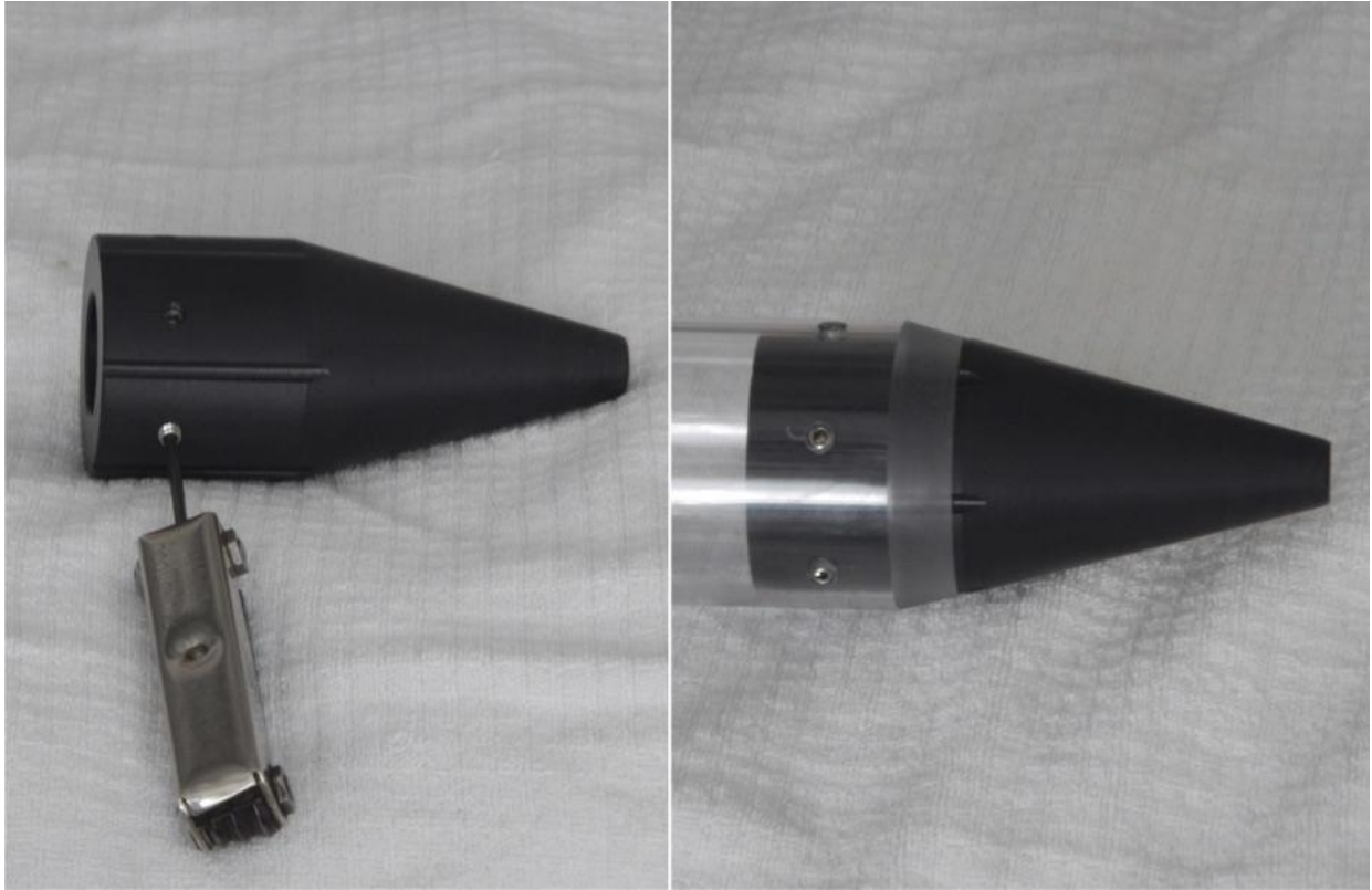
Figure 4. End cap with one set screw out in the “lock” position (left) and end cap installed in towing position with all set screws out in the “lock” position (right). Note that the 15° taper on the end of the tube matches the end cap.
