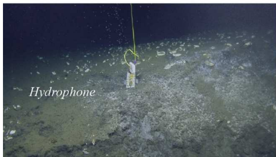
393 Figure 2: (a) Remotely Operated Vehicle pictures of hydrophone and float in a field of bubble 394 streams at the SW Heceta Bank seep site shown in Figure 1. (b) Schematic showing flow of 395 methane bubbles from sub-seafloor conduits into the water-column (based on Minneart, 1933). 396 Oscillation of bubbles caused by detachment at the seafloor conduit leads to sound production.
