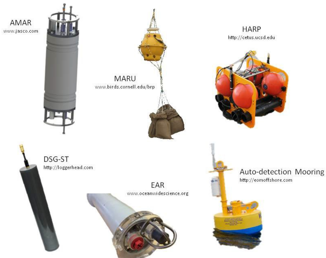
Figure 2. Fixed autonomous recorders for passive acoustic monitoring of marine mammals.
