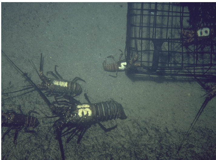
Hawaiian spiny lobsters held at the Kewalo Research Facility were used to test the optimal placement of escape vents that would retain legal sized animals yet let undersized individuals escape.
