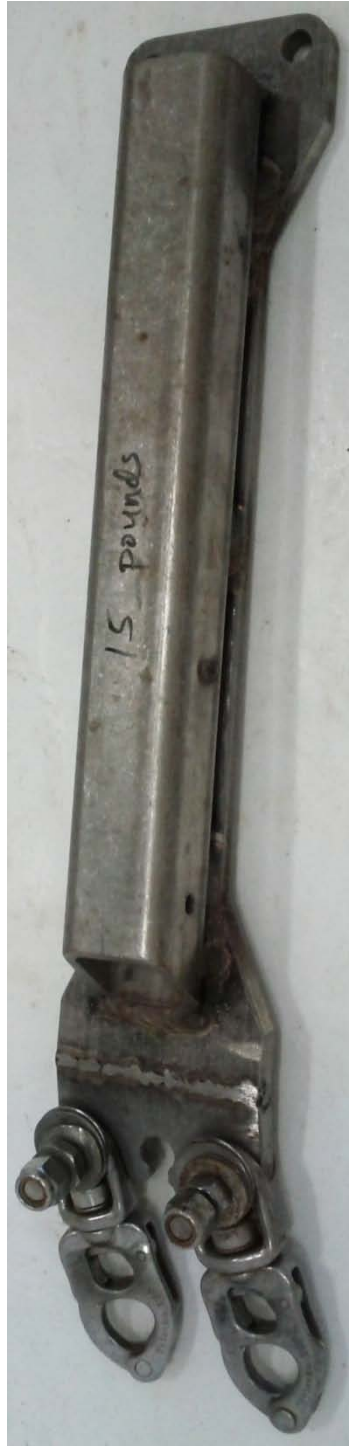
Figure 2f. - - The bottom contact sensor and its footrope attachment configuration to the ground gear used during the 2012 EBSS survey.
