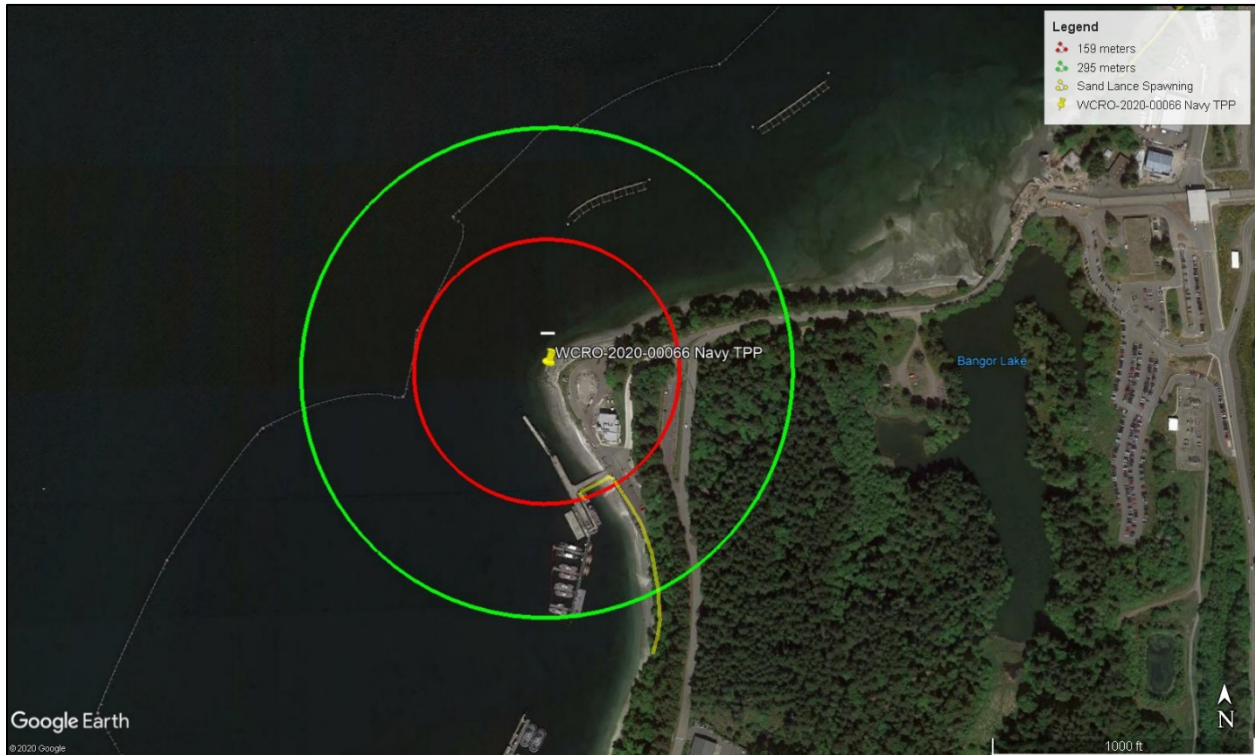
Figure 16: Forage fish and impact pile driving
