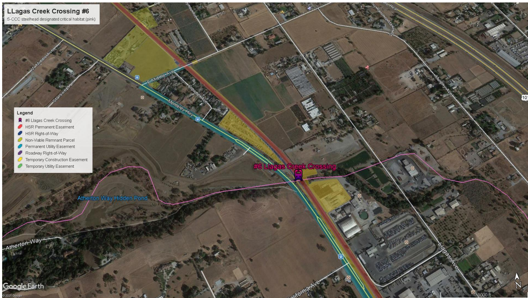
Figure 20. Llagas Creek crossing #6 by HSR elevated viaduct and ROW (red/dark blue) with temporary construction easement estimates (yellow) relative to S-CCC steelhead designated critical habitat (pink line) near Atherton Way Hidden Pond and Monterey Highway. Electrical interconnections/road re-route in teal.
