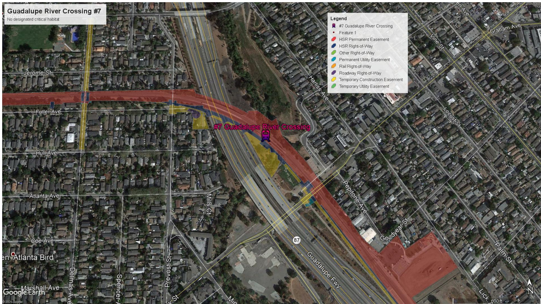
Figure 24. Close-up of Guadalupe River crossing #7 by HSR elevated viaduct, ROW, and permanent buildings (red/dark blue) with temporary construction easement estimates (yellow). No CCC steelhead designated critical habitat in the section of river crossed near Highway 87/Guadalupe Freeway.
