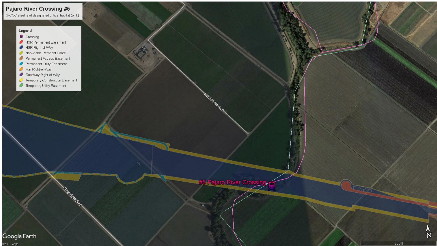
Figure 18. Close-up of Pajaro River crossing #5 by HSR elevated viaduct/berm and maintenance facility ROW (dark blue) with temporary construction easement estimates (yellow) relative to S-CCC steelhead designated critical habitat (pink line). Electrical interconnections in teal.
