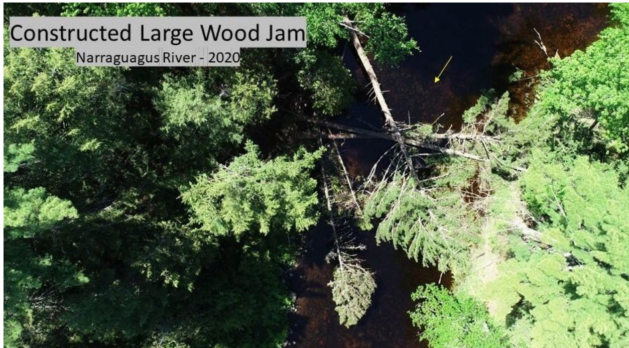
Figure 5.3.6. Large wood jam created using 3 larger trees, and 2 smaller trees ; felled manually using a Griphoist, Narraguagus River (2020). (photo credit: Chris Federico, Project SHARE)
