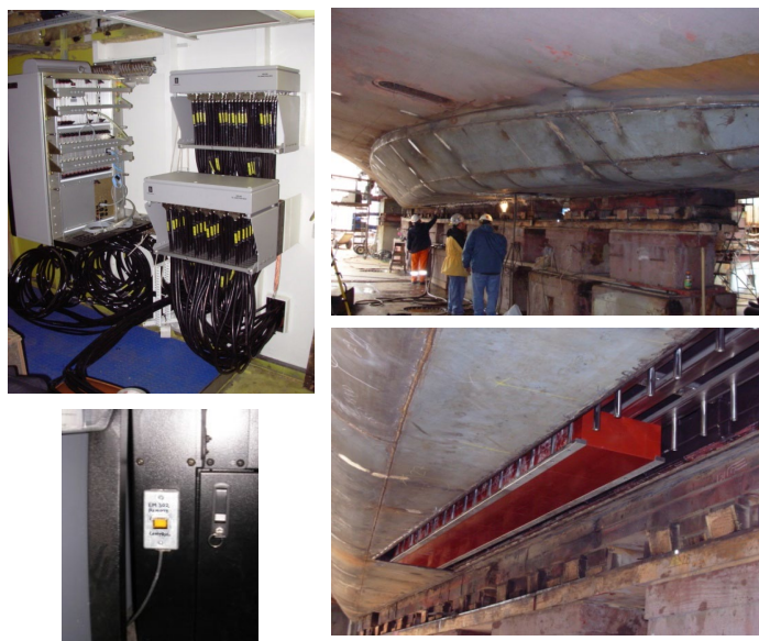
Figure 4. EM302 hardware (Clockwise from left) EM 302 Transmit Receive Unit (TRU) unit, transducer fairing, elements of EM 302 being installed inside the fairing, and the TRU remote on/off switch.
