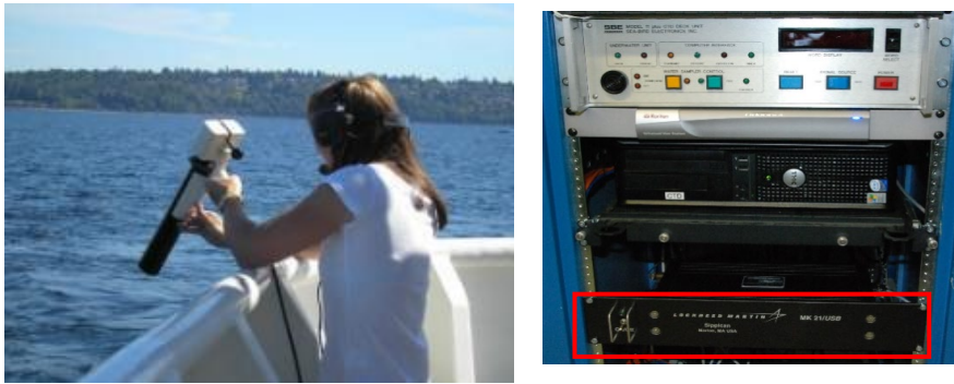
Figure 8. Sippican XBT launch setup from the aft deck (left). Deck unit for Sippican XBT (right).
