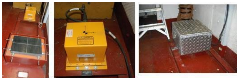
Figure 5. POS MV hardware. From left to right: IMU and granite block, IMU, and the IMU under protective housing.
