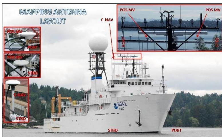
Figure 6. The arrangement of the miscellaneous antennas onboard , including the Civil Navigation (CNAV) GPS antenna and the POS MV port and starboard antennas.
