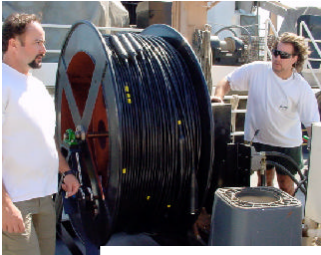
Illustrations of the towed 5-element hydrophone array and signal monitoring trackin the g laboratory survey.
