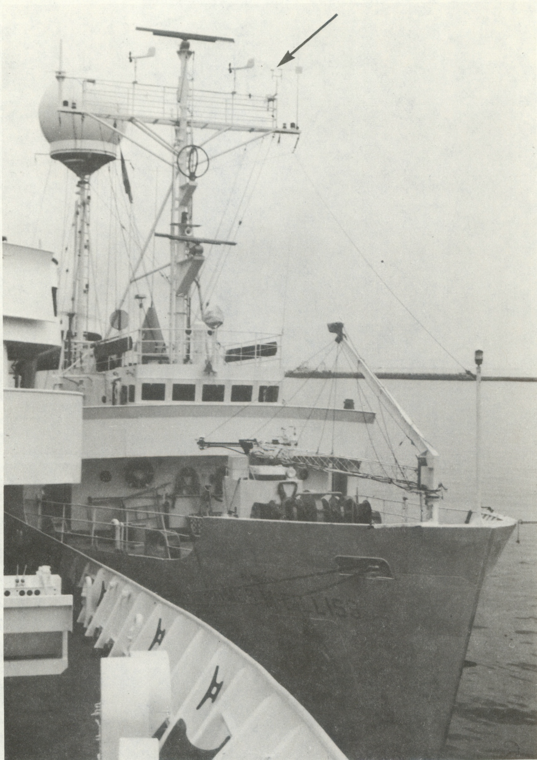
Figure 4.--Location of mast wind sensors on the Gilliss .
