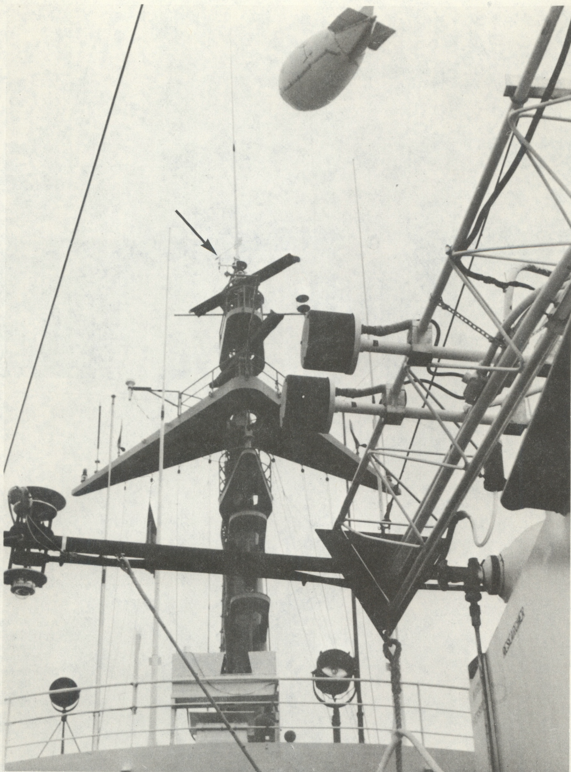
Figure 3.--Location of mast wind sensors on the Researcher .
