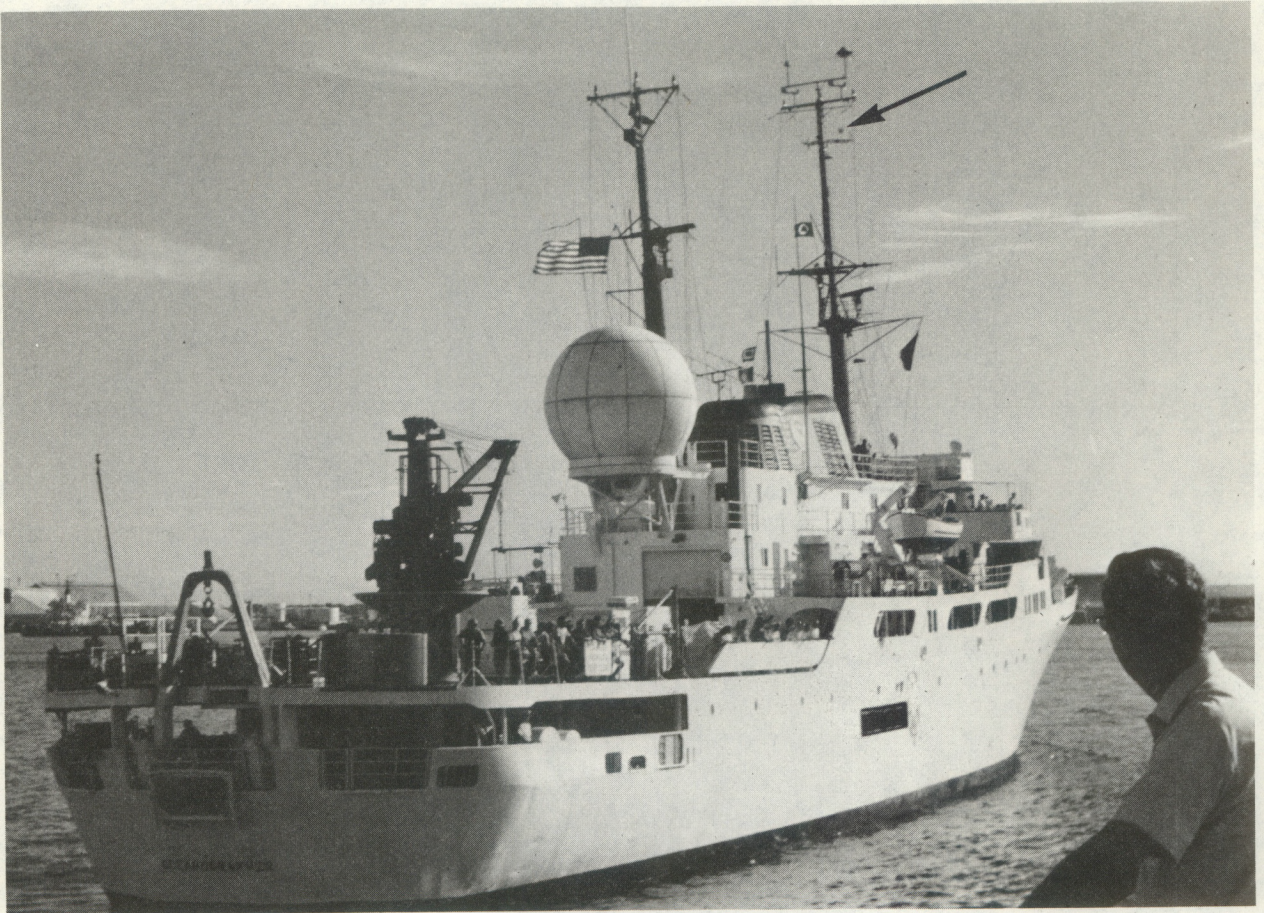
Figure 6.--Location of mast wind sensors on the Oceanographer .
