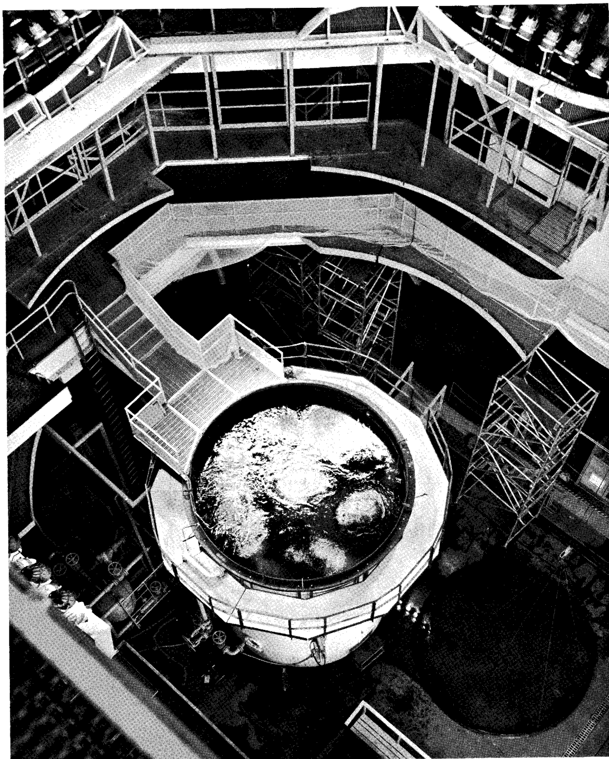
Figure 15. The 27,000-gallon fish-sensor testing tank at the Mississippi Test Facility. The tank is 15 feet in diameter, 22 feet high, and is supplied with filtered oxygenated fresh water. A crane is used to transfer fish from nearby holding tanks. The device resembling an inverted parachute is one of the two screens used to restrict target fish to a particular depth level. Tungsten lamps at the top of the picture supply light at about 60 percent the intensity of sunlight.
