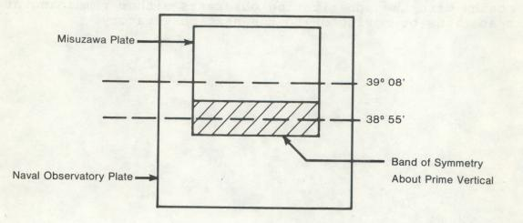
Field of Naval Observatory's PZT compared to field of Misuzawa's PZT
