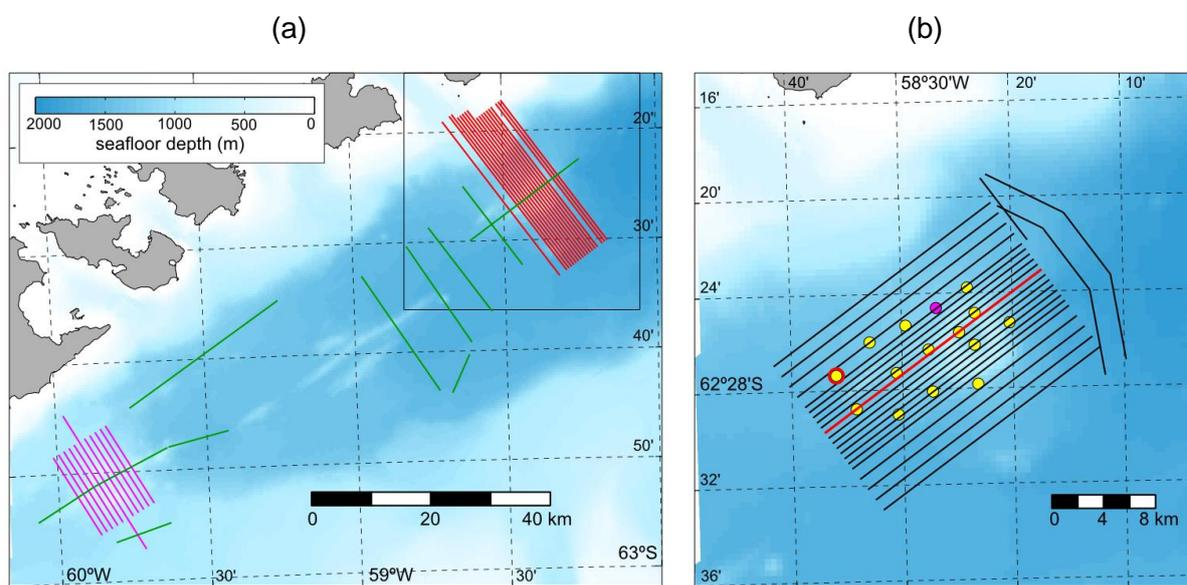
Figure 6. (a) MCS profiles carried out over Orca volcano (red), Humpback volcano (purple), and in the Bransfield rift (green). (b) Shooting profiles carried out over the seismic instruments surrounding Orca volcano (black), for tomography and refraction studies. The shots of the profile marked in red, recorded at the OBS encircled in red, are displayed in Figure 15. The area zoomed in (b) is marked by a black box in (a).
