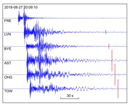
Figure 7. Seismograms (vertical component) of a M5.6 tectonic earthquake recorded by land seismometers in the Bransfield Strait area on August 27, 2018. Data are normalized to their maxima; the red bars on the right side indicate the relative seismogram amplitudes. The start time of the records is indicated at the top left.
