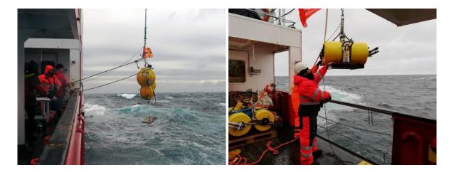
Figure 3b. Deployment of broadband (left) and short-period (right) OBS during the BRAVOSEIS 2019 cruise.
