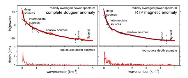
Figure 13. Radially-averaged power spectra and estimate of top source depth of the anomaly sources. (left) Complete Bouguer anomaly. (right) Reduced-to-pole geomagnetic anomaly.
