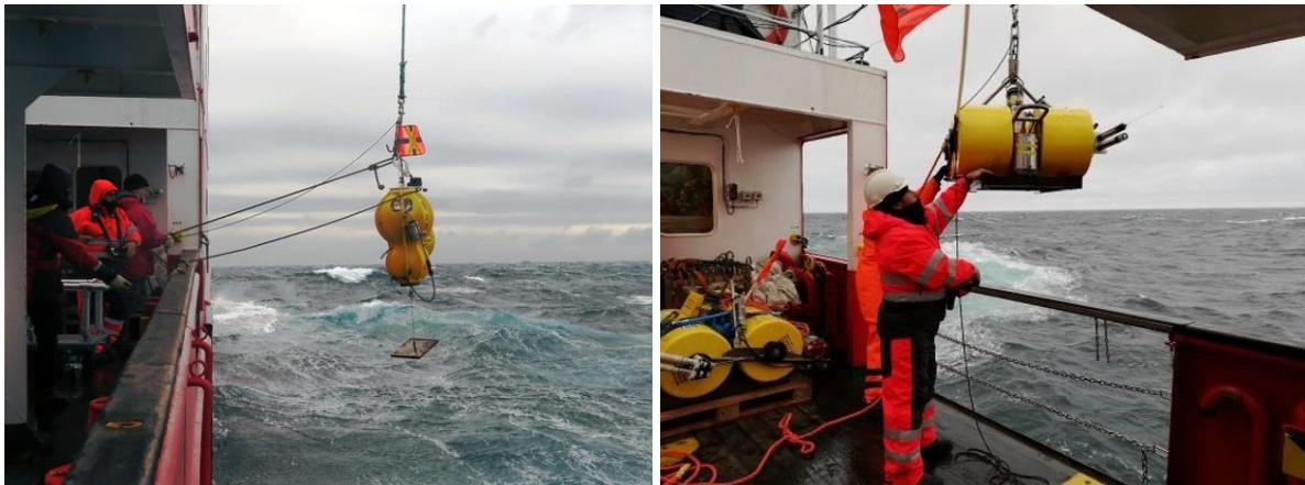
Figure 3b. Deployment of broadband (left) and short-period (right) OBS during the BRAVOSEIS 2019 cruise.
