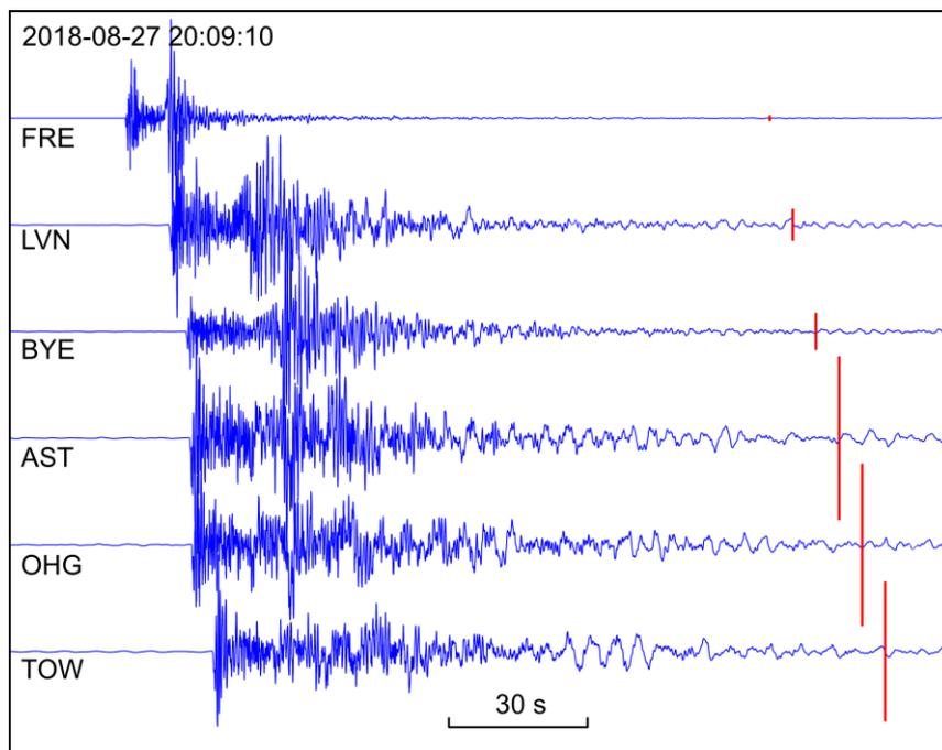
Figure 7. Seismograms (vertical component) of a M5.6 tectonic earthquake recorded by land seismometers in the Bransfield Strait area on August 27, 2018. Data are normalized to their maxima; the red bars on the right side indicate the relative seismogram amplitudes. The start time of the records is indicated at the top left.
