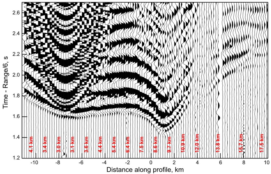
Figure 15. Example record section plotted with a reduction velocity of 6 km/s for shots along a tomography line, recorded on a short-period OBS (BRA13, see Figure 6). The data have been filtered with a 5 Hz, 4th-order, high-pass filter and are scaled with range. The horizontal axis shows the shot position along the profile and the red labels indicate the range of the shots.
