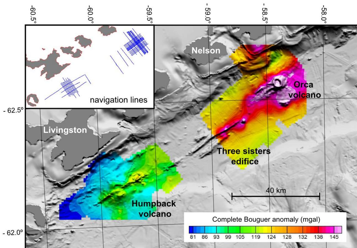
Figure 11. Complete Bouguer anomaly map of the Central Bransfield Basin using data from the BRAVOSEIS cruises. Grey-shaded background is a digital elevation model combining GMRT and multibeam data. The inset shows the navigation lines after processing. See color legend form interpretation.
