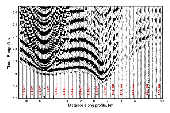
Figure 15. Example record section plotted with a reduction velocity of 6 km/s for shots along a tomography line, recorded on a short-period OBS (BRA13, see Figure 6). The data have been filtered with a 5 Hz, 4th-order, high-pass filter and are scaled with range. The horizontal axis shows the shot position along the profile and the red labels indicate the range of the shots.
