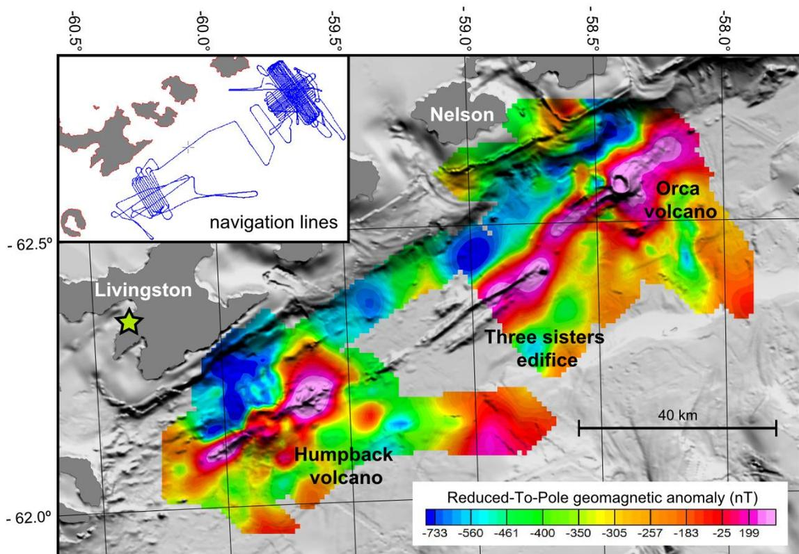
Figure 12. Same as Figure 11 for the reduced-to-pole geomagnetic anomaly map of the Central Bransfield Basin. The star shows the location of the permanent geomagnetic station at Livingston Island.
