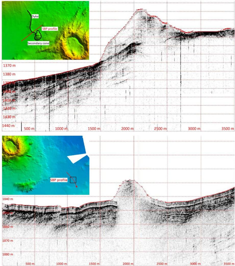
Figure 10. Examples of the sediment profiler data over two selected targets: a volcanic fissure (top) and a mud volcano (bottom). The insets show the positions of the SBP profiles relative to Orca volcano.
