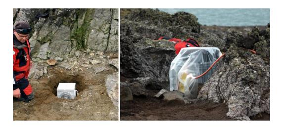
Figure 3a. (left) Installation of a land seismometer inside a buried protecting case at Snow Island. (rigth) Final aspect of the battery pack and acquisition system of station PEN at Penguin Island (height ~0.6 m).
