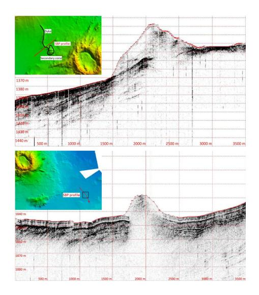
Figure 10. Examples of the sediment profiler data over two selected targets: a volcanic fissure (top) and a mud volcano (bottom). The insets show the positions of the SBP profiles relative to Orca volcano.
