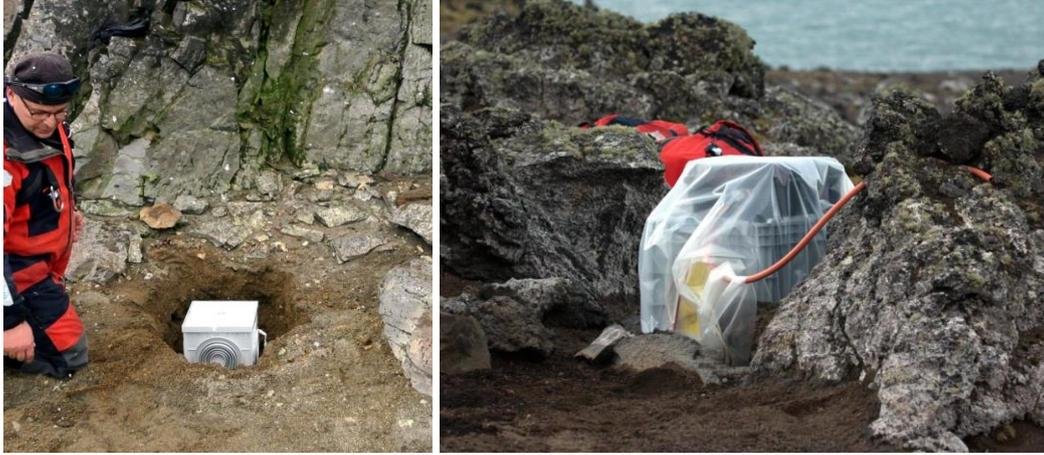
Figure 3a. (left) Installation of a land seismometer inside a buried protecting case at Snow Island. (right) Final aspect of the battery pack and acquisition system of station PEN at Penguin Island (height ~0.6 m).
