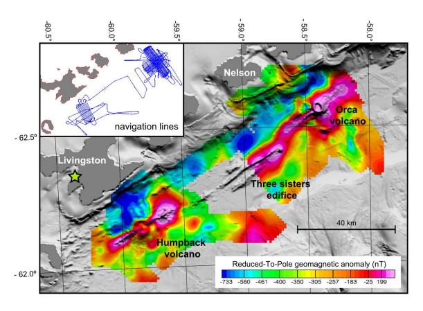
Figure 12. Same as Figure 11 for the reduced-to-pole geomagnetic anomaly map of the Central Bransfield Basin. The star shows the location of the permanent geomagnetic station at Livingston Island.
