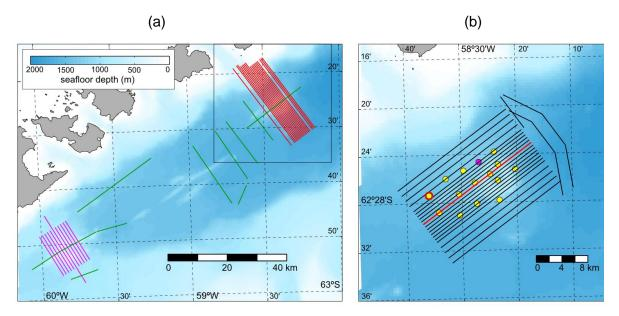
Figure 6. (a) MCS profiles carried out over Orca volcano (red), Humpback volcano (purple), and in the Bransfield rift (green). (b) Shooting profiles carried out over the seismic instruments surrounding Orca volcano (black), for tomography and refraction studies. The shots of the profile marked in red, recorded at the OBS encircled in red, are displayed in Figure 15. The area zoomed in (b) is marked by a black box in (a).
