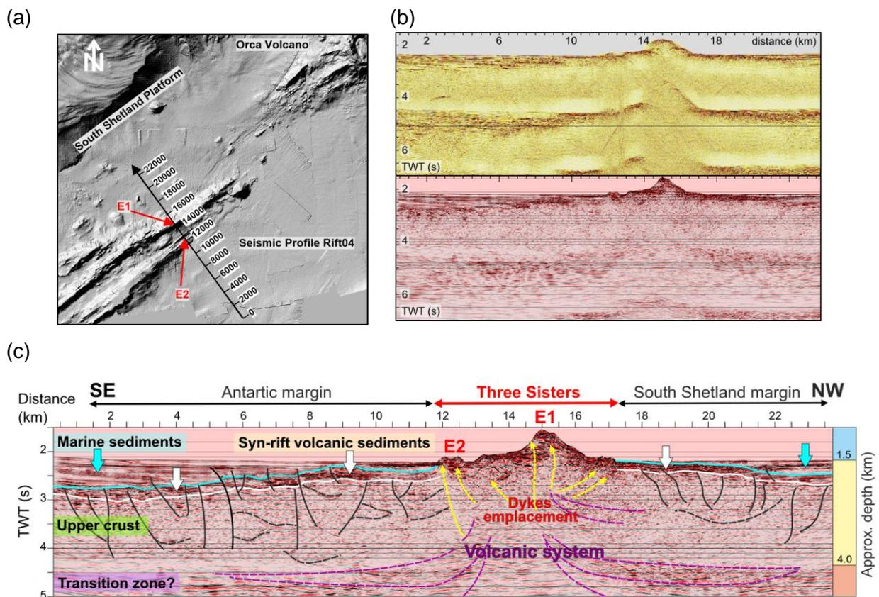
Figure 14. (a) Location of the seismic profile on the NE part of the Three Sisters structure. The profile is ~24 km long, and crosses above two of the main ridges in a direction perpendicular to the rift. (b) Brute stack of seismic profile (top) and result of processing algorithms that reduce the amplitude of multiples (bottom). (c) Resulting seismic section, where we highlight the main velocity contrasts and display a preliminary interpretation.
