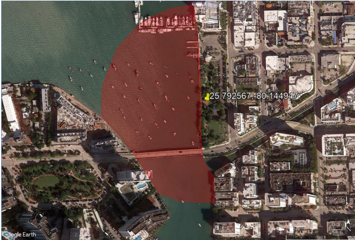
Figure 4. Image showing the action area (within the red circle having a 705-ft radius) defined by the extent of behavioral noise effects based on the proposed action’s installation of 14-in concrete piles using impact hammer (©2020 Google).
