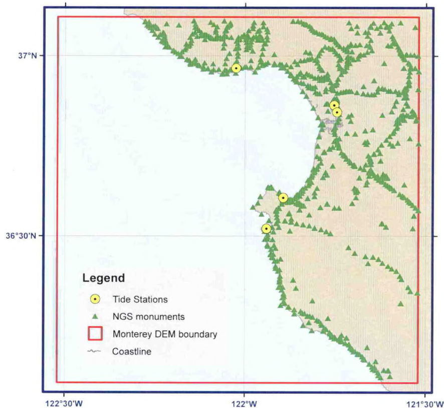
Figure 22. Location of NGS geodetic monuments, shown as green triangles, and the NOAA tide stations, yellow circles. NGS monument elevations were used to evaluate the DEM.
