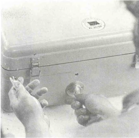
Figure 13.--Tag injection sequence while using optional step of passing fish by hand to injector operator. As fish in operator's right hand is placed in headmold and the injector is activated by foot switch, a second fish is placed into left hand of operator. When injector cycle is finished, operator places fish in his right hand into funnel of the quality control device about 10 inches to the right of operator's hand. The fish in left hand is now transferred to the right hand with minimal movement. During this transfer from the left to the right hand, the fish is gently rolled 180° so that its head is in proper alignment and close to the headmold of the injector.
