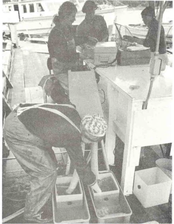
Figure 15.--As fish pass through the quality control device, tags are magnetized and verified. Improperly marked fish are sorted into separate containers. Note in this sequence that no one is passing fish to the tag injector operator and he is retrieving the next fish to be tagged from anesthetic with his left hand.
