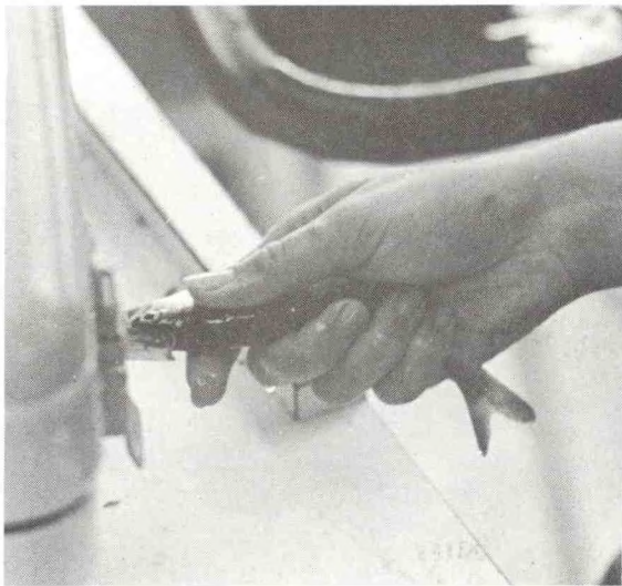
Figure 14.--Coho smolt in headmold of tag injector during injection sequence.
