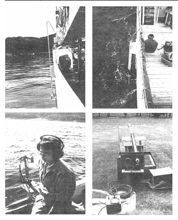
Figure 4. Hydrophone and pole rotating system.
