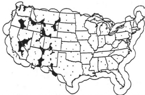
Figure 2. WSR-88D network coverage at 10,000 feet above site level for the contiguous United States. Hatched regions represent areas not covered below 10,000 feet. Dots represent locations of radar towers.
