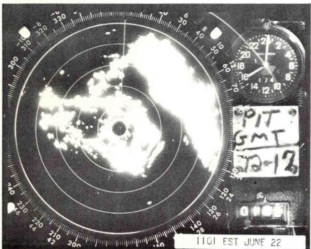
Pittsburgh, Pennsylvania, radarscope photographs. Some of the holes appearing in the echoes are contours of heavy rain created by the Video Integrator and Processor mode of the radar set. Note the slow movement of the rain patterns. (Range markers: 25 miles).
