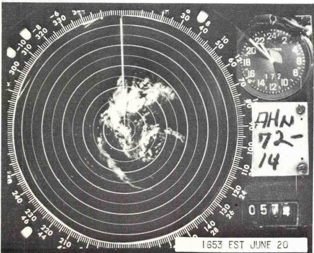
Athens, Georgia, radarscope photographs. Movement of rainshield is evident; echoes near the vortex can be seen faintly. (Range markers: 50 miles, heavy; 25 miles, lighter).
