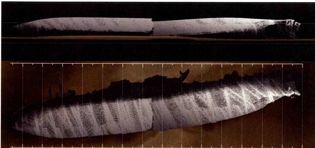
Figure 4-3: High-resolution multibeam survey with visualization software of inverted tanker torpedoed off the coast of North Carolina in 1942 (Image generated by ADUS and courtesy of NOAA).
