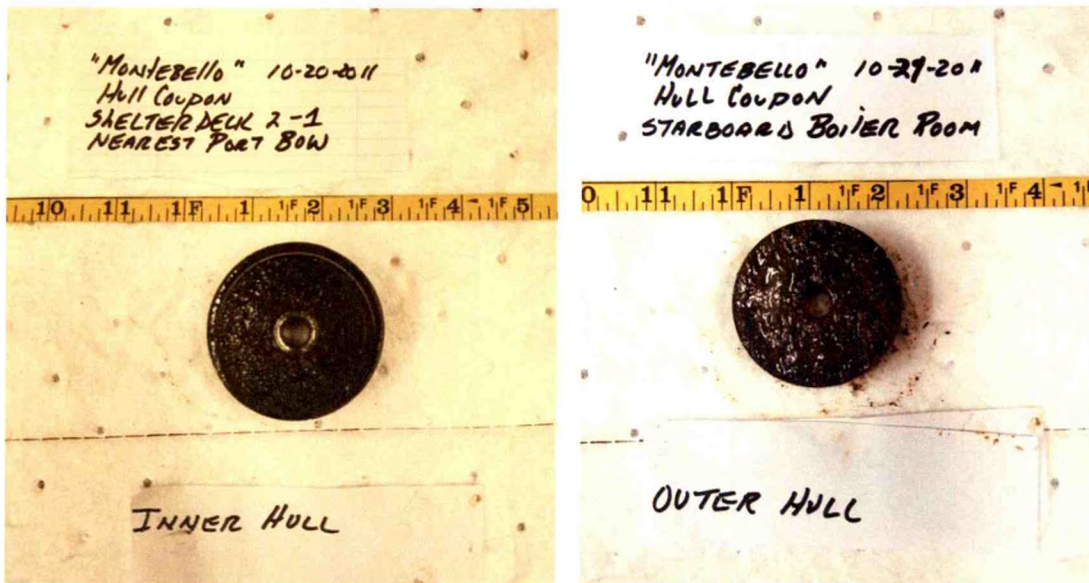
Figure 2-4. Two of coupon samples from the SS Montebello prior to analysis.
