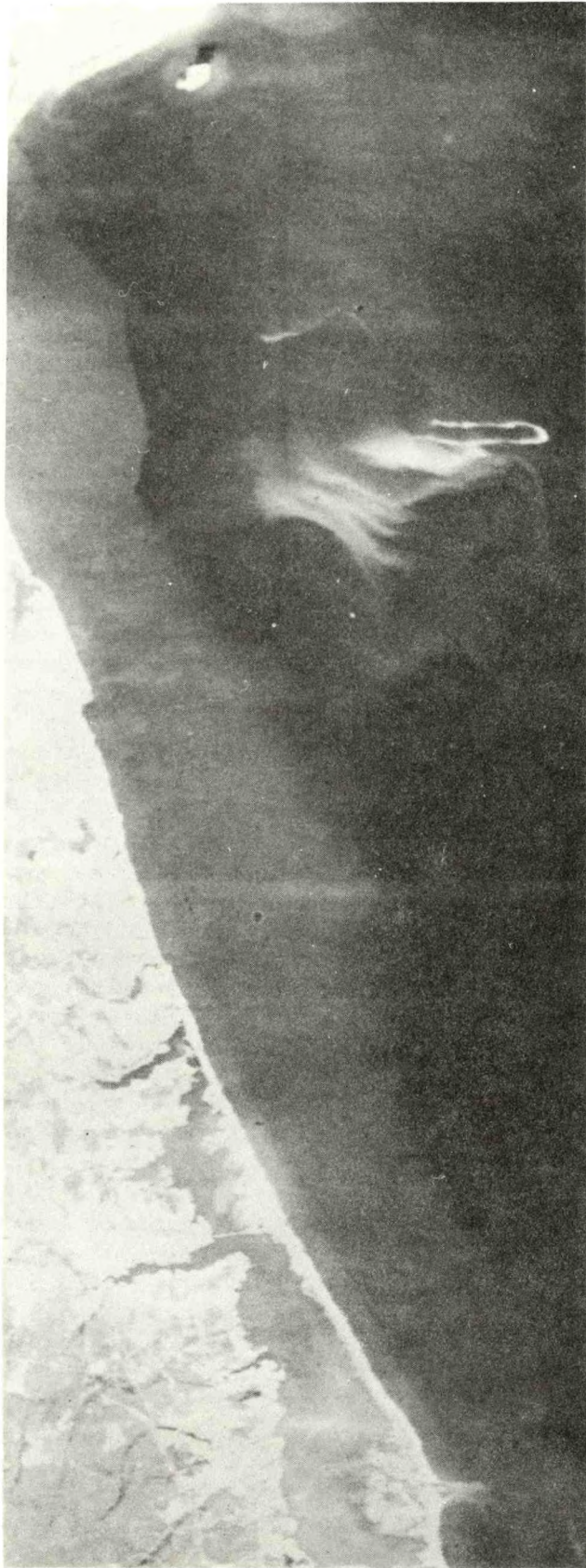
Figure 6.--Enhanced scanner image of New York Bight, April 9, 1975--portion of shore of Long Island and New Jersey shore from Barnegat Inlet to just south of Sandy Point. Newly dumped acid waste is sharp "U". Earlier dumped acid drifts and diffuses to the west. This westward drift is characteristic of nearly all imagery for this area. The square shaped pattern north of the acid waste is a sewage sludge dumpsite. The bright area along the New Jersey shore is the normal flow pattern of Hudson River plume. The high relative reflectivity of the plume is due to the relatively high particulate load where the Hudson River discharges. (Source: National Oceanic and Atmospheric Administration)
