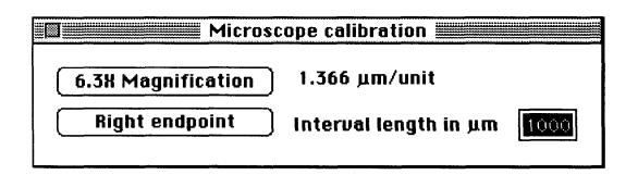
Figure 10 Enter the number of  $\mu m$  read and click on the **Right endpoint**. The program will automatically calculate the number of  $\mu m$  / unit.
