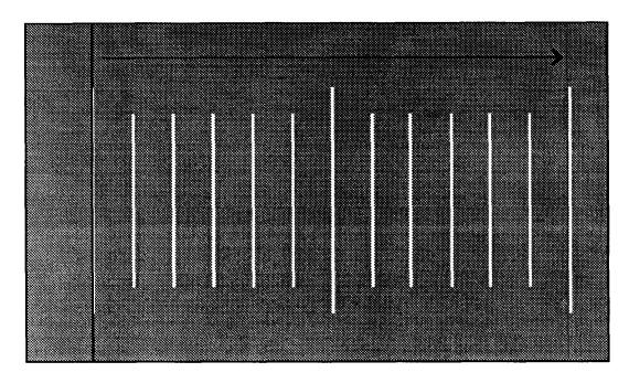
Figure 9 Moving the HEI crosshair to the left end of a stage micrometer, the arrow indicates moving the crosshair to the right endpoint.
