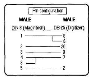
Figure 58 Wiring schematic for cross-overs in the DIN-8 to DB25 cable connecting the Macintosh to the HEI digitizer.
