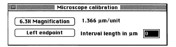
Figure 8 Place the cursor at the left end of the micrometer and click on **Left endpoint**.
