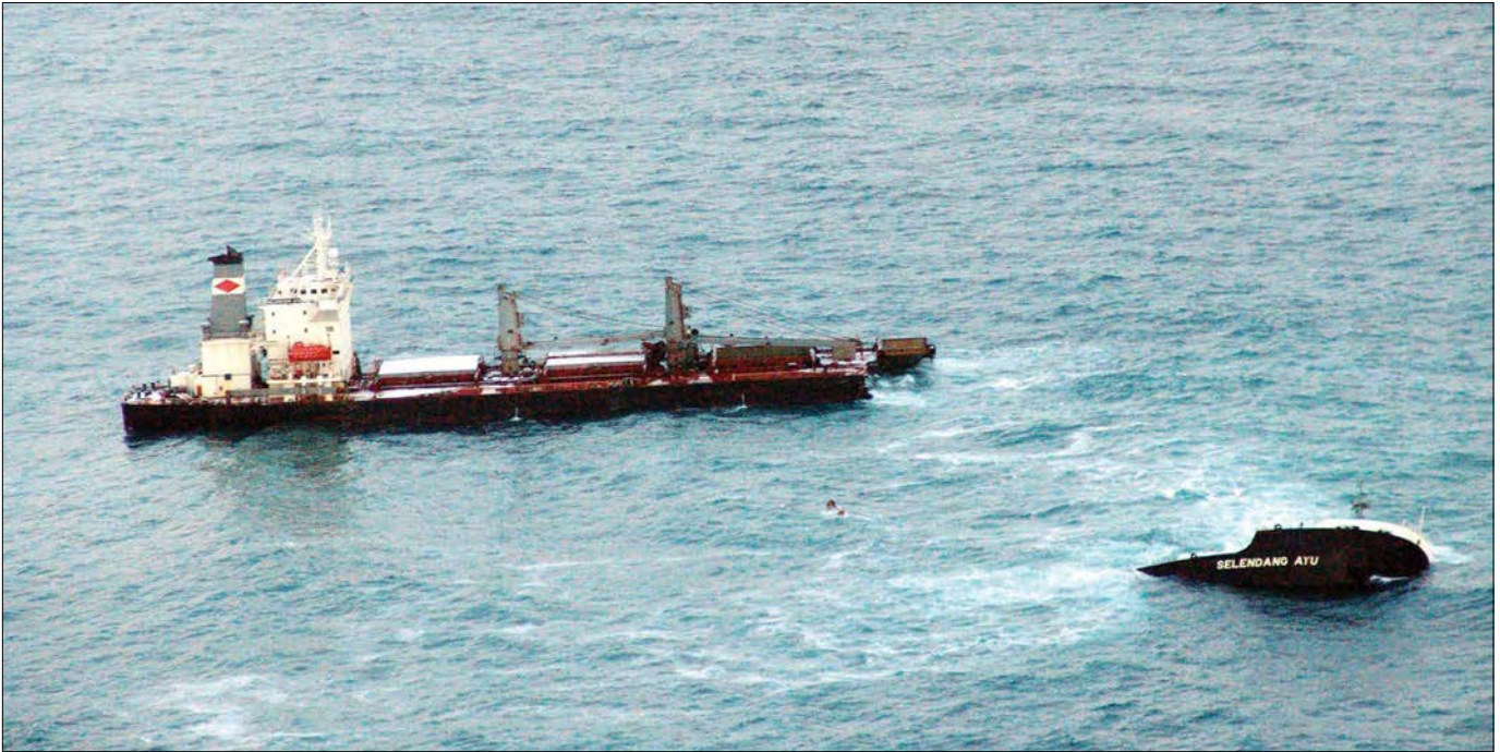
After splitting in two near Unalaska Island, Alaska, in December 2004, the Selendang Ayu 's bow began to submerge due to weather conditions. When the vessel split, its fuel tanks leaked more than 300,000 gallons of fuel into the Arctic ocean. Coast Guard photo
