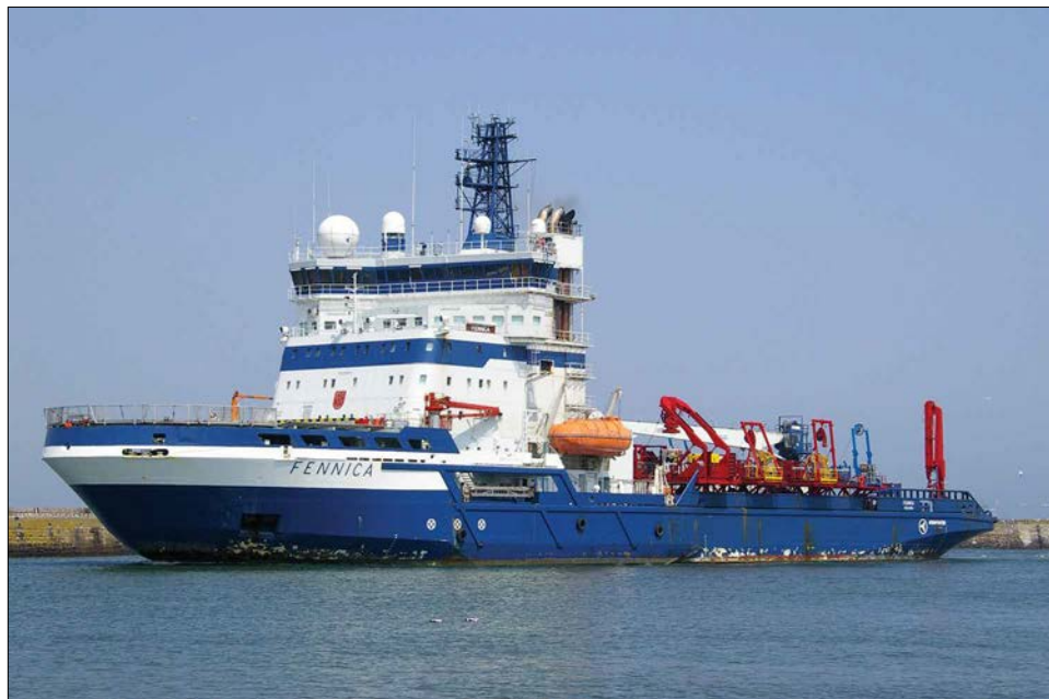
On July 2015, Fennica , a specially built Finnish ice-classed, multi-purpose vessel, was underway with a pilot aboard, near Unalaska Bay in the Aleutian Islands when it grounded on a rock not reflected in the waterway's most current nautical chart. Post-grounding surveys of the area would identify several locations shallower than reported on the relevant National Oceanic and Atmospheric Charts. Photo courtesy of James Dodds
