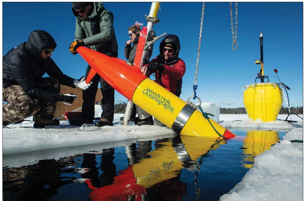
The Arctic Domain Awareness Center's leading research project, the propeller-driven Long-Range Autonomous Underwater Vehicle system, undergoes testing in a controlled environment. The system is designed to advance domain awareness and can be one solution to address significant oil spills in Arctic waters. Photo courtesy of The Arctic Domain Awareness Center
