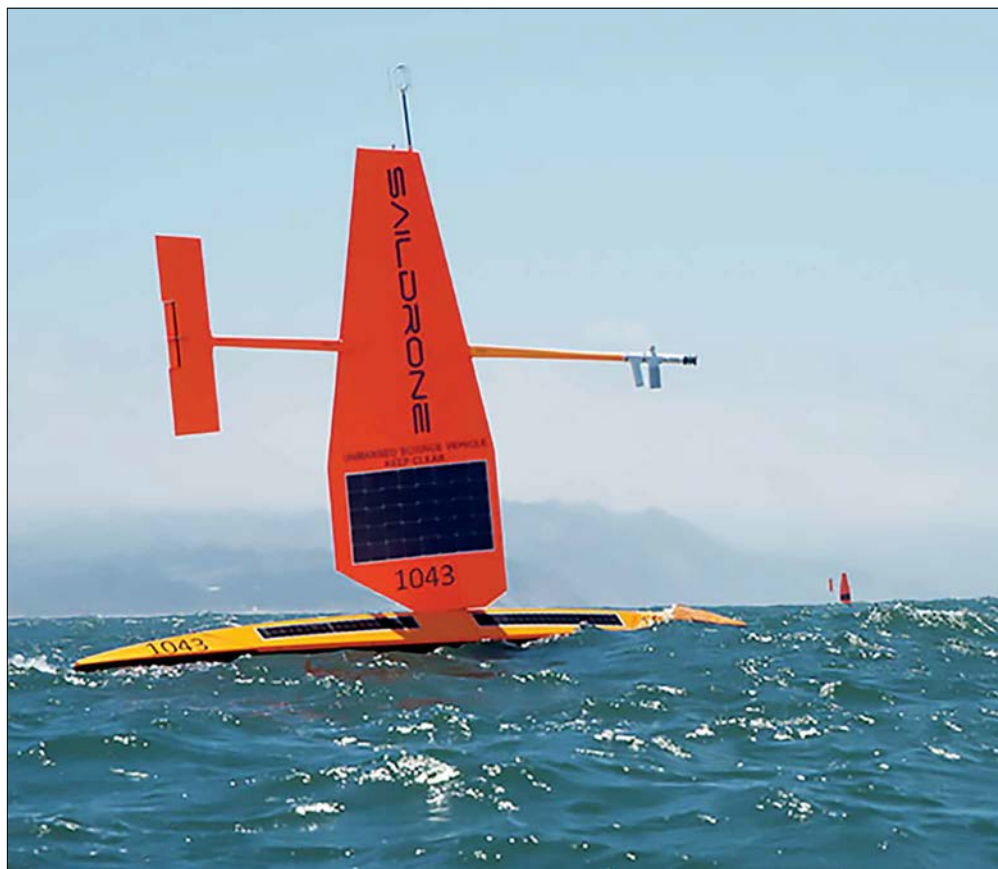
Just west of the Golden Gate Bridge, saildrones begin their journey to the Bering Sea in May 2020. The mission was part of a 2020 partnership between the National Oceanic and Atmospheric Administration and Saildrone, Inc., to capture survey data in the Bering Sea. Saildrones are a fleet of wind and solar-powered ocean drones that monitor the state of the planet in real time, above and below the surface. Photo courtesy of Saildrone, Inc.
