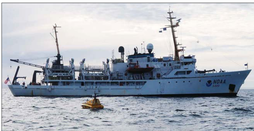
National Oceanic and Atmospheric Administration Ship Fairweather launches the unmanned surface vehicle BEN, or Bathymetric Explorer and Navigator, in July 2018 to collect Arctic hydrographic survey data. Vehicles like BEN help counter the logistical challenges of operating and researching in the Arctic. Photo courtesy of National Oceanic and Atmospheric Administration
