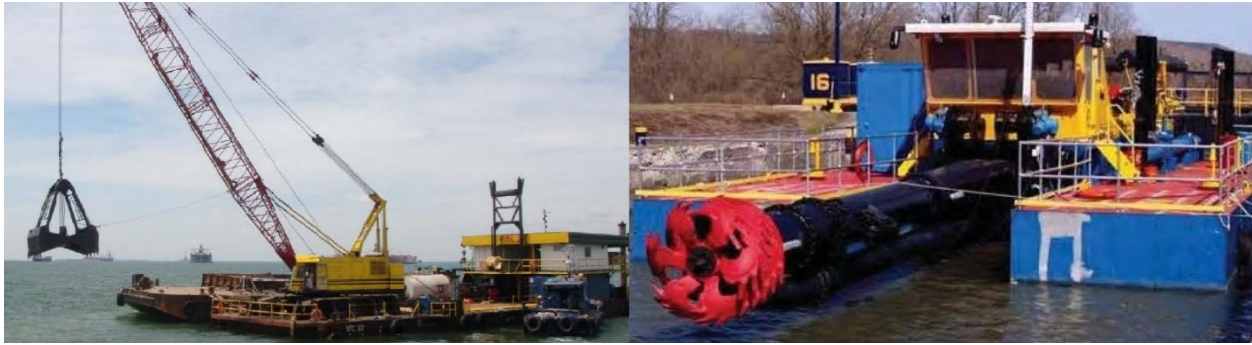
Figure 2. Mechanical and hydraulic dredges. The left image shows a mechanical dredge with a clamshell bucket and a sediment transport barge tied alongside. The right image is a hydraulic dredge with a cutter-head.
