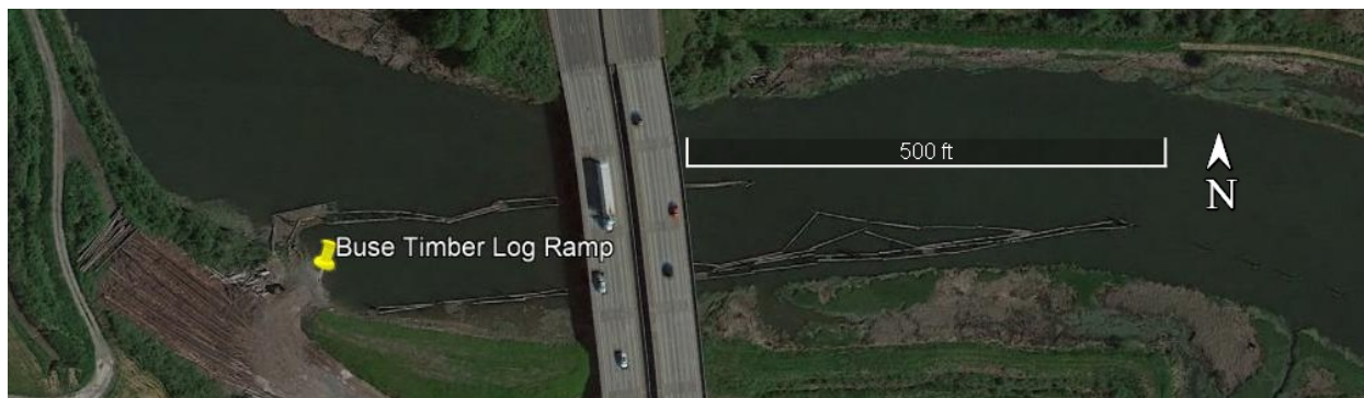
Figure 4. Google satellite image of the Buse Timber & Sales Inc. log ramp on Union Slough, just west of the I-5 Bridge, showing two lines of logs moored to piles in the channel.
