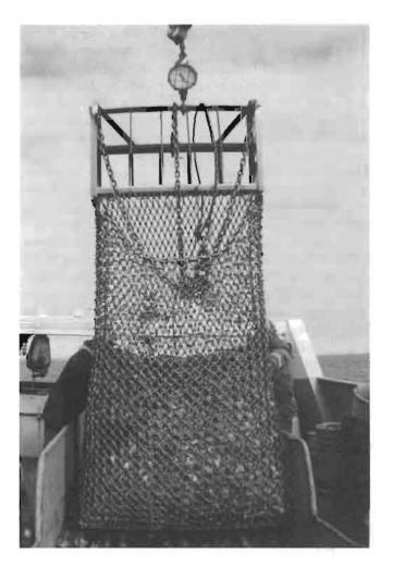
Figure 5 A 500 kg catch of live scallops taken in a 1.5 m Breidafjördur dredge during a research survey.
