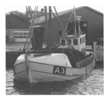
Figure 3 An old traditional Danish mussel vessel carrying around 30 t of mussels.
