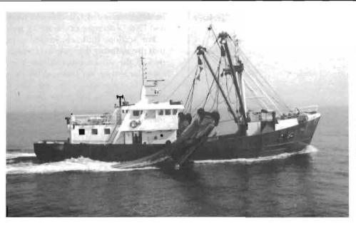
**Figure 9** Flatfish-directed beam trawler (30 m length over all, 182 GRT, 900 HP) of the type currently fishing in the North Sea and on the western grounds. Photograph by R. Fonteyne.
