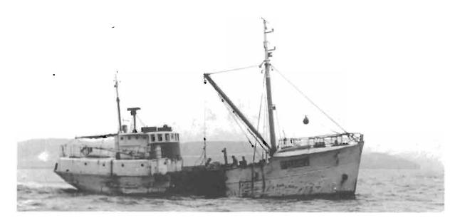
Figure 3 An older fishing vessel used for dredging scallops.
