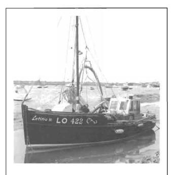
**Figure 10** A cockle dredger fitted with hydraulic suction gear. Photograph by the author.
