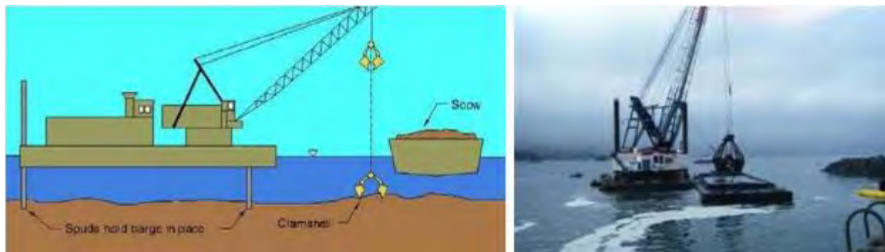
Figure 3. Typical clamshell dredge schematic (left) and photograph (right). 1
