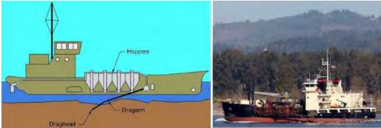
Figure 1. Typical hopper dredge schematic (left) and the Yaquina hopper dredge (right).
