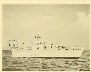
GENERAL DESCRIPTION: Canabilities—General coastal oceanographic sampling, benthic dredging, gill net fishing, 2nd limited trawling Hull style—VEE, planning cruiser Number of masts—1, for navigation lights only Construction material—Mahogany Method of fabrication—Bottom double, sides batten Screw type: Number of blades-3 Fixed pitch or CP-Fixed, 21"×21" RH + LH
